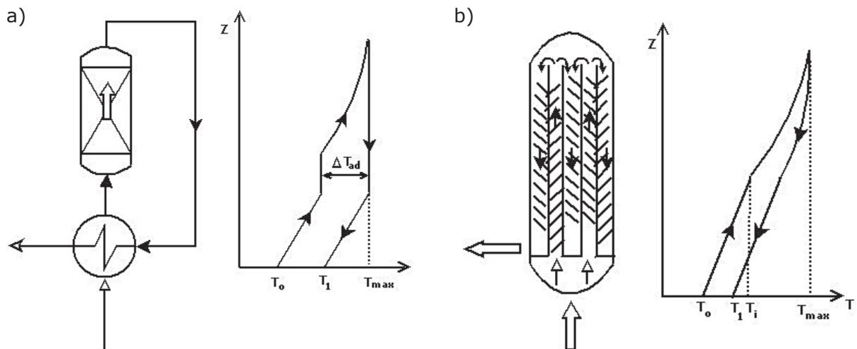
**Fig. 1.** The schemes of construction and typical temperature courses of monolith reactors (CMR): a) classical and b) reverse flow;  $T_o$  – input temperature,  $T_i$  – initiation temperature,  $T_{max}$  – maximum temperature,  $T_l$  – output temperature,  $\Delta T_{ad}^1 = T_l - T_o$  [2]
