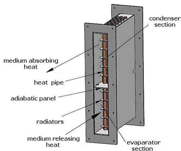
Fig. 3. Single section of the “heat pipe” exchanger
