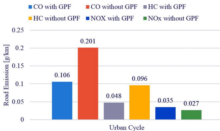
Fig. 7. Road emission results of gaseous exhaust components in the urban section
