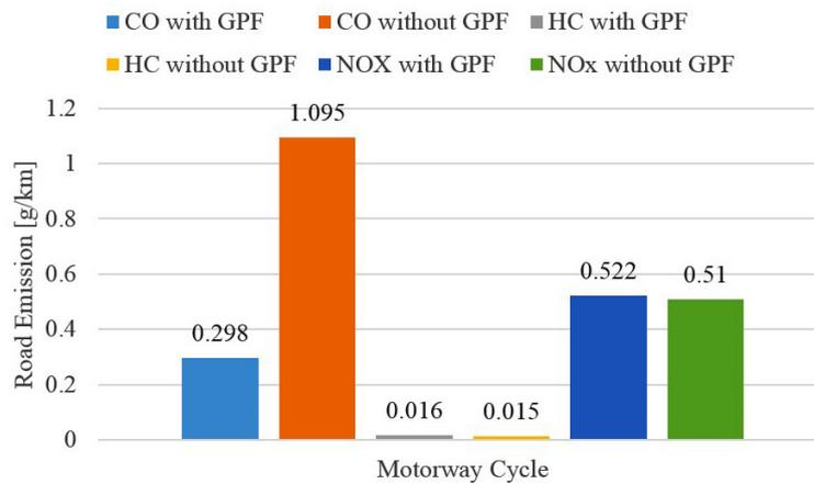
Fig. 9. Road emission results of gaseous exhaust components in the highway section
