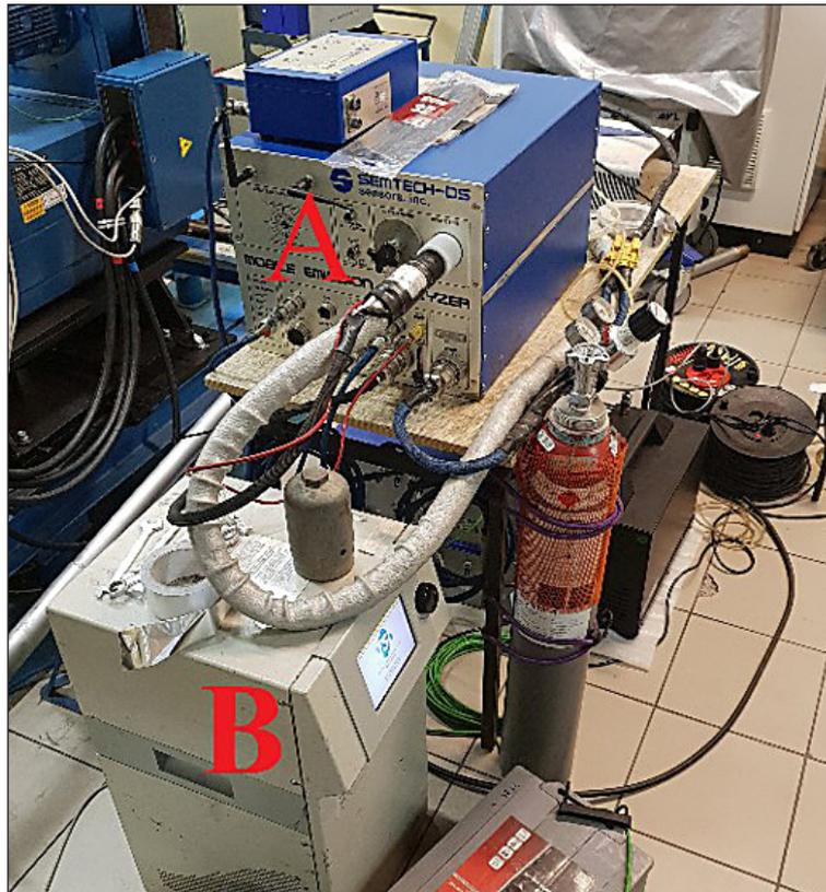
Fig. 5. PEMS apparatus during the calibration process: A) SEMTECH DS, B) EEPS TSI
