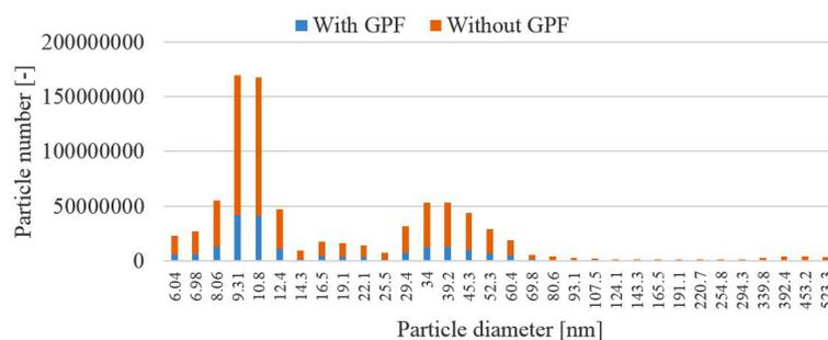
Fig. 11. Particulates size distribution during tests with and without particulate filter
