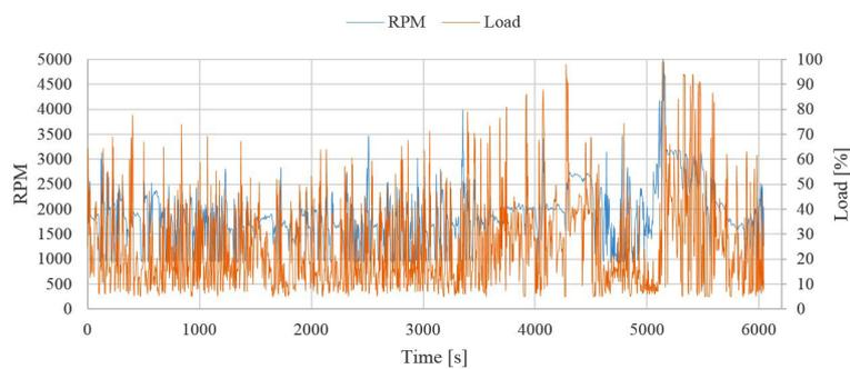
Fig. 6. RPM and load of the engine during test
