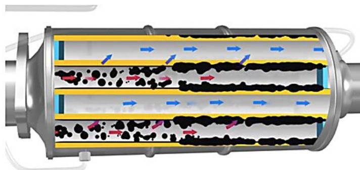
Fig. 2. Particulate filter principle of operation [Semtech 2000]
