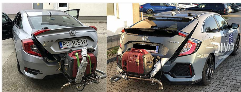
Fig. 3. View of tested vehicles with testing equipment: A) vehicle without GPF, B) vehicle with GPF
