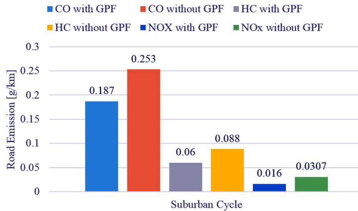
Fig. 8. Road emission results of gaseous exhaust components in the rural section
