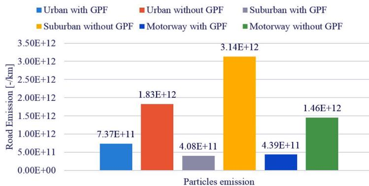
Fig. 10. PN emission during tests with and without GPF
