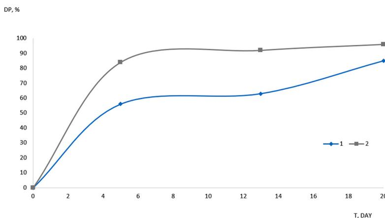
Fig. 3. The comparative sorption capacity of the bio-plateau without options (1) (2) additional aeration, C<sub>0</sub> (Cd) = 1 mg/l
