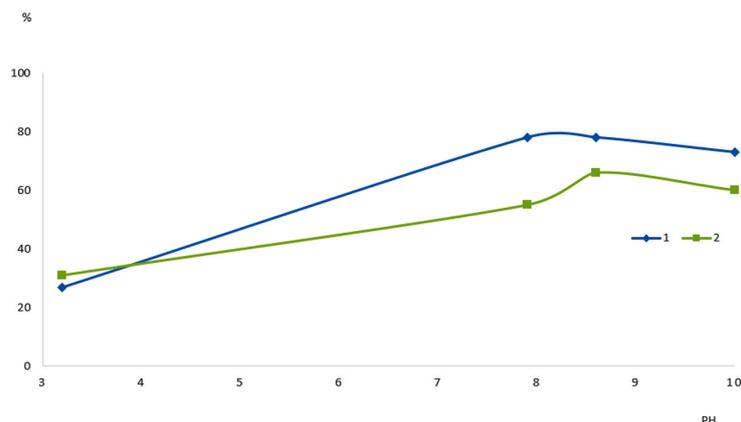
**Fig. 4.** Correlation between the degree of purification from cadmium ions (CO – 1) and the degree of transpiration (CT – 2) on the 15th day of observation depending on the pH of the incubation environment
