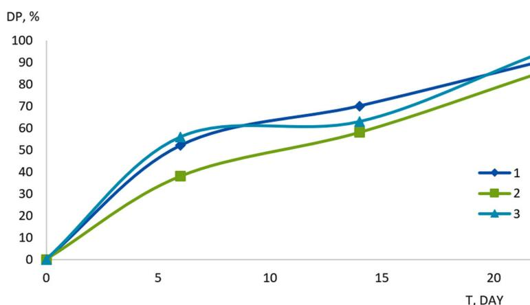
Fig. 2. Comparison of sorption capacity of plants with respect to cadmium (II) ions, C<sub>0</sub> = 1 mg/l: 1 – barley, 2 – oats, 3 – rye
