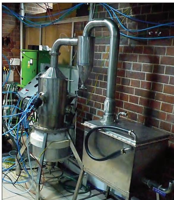
Fig. 4. Elements of installation for plasma processing of waste
