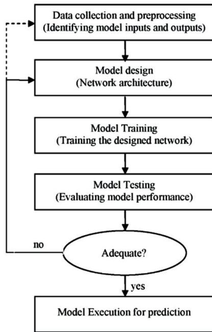
Figure 3. A step-by-step model creation procedure [Güçlü and Sükrü, 2010]
