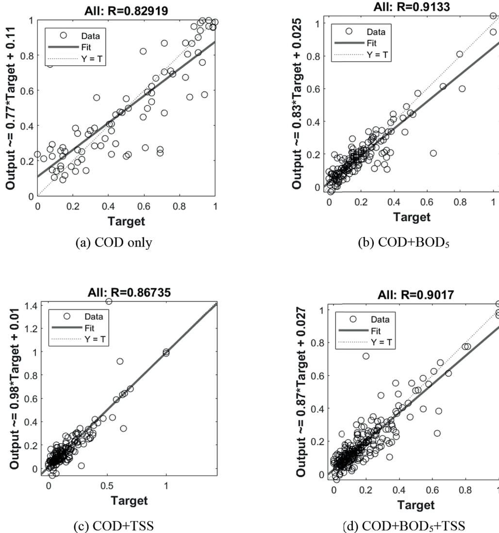
**Figure 4.** Correlation between COD prediction model results and actual data: (a) MISO, (b, c and d) MIMO Models
