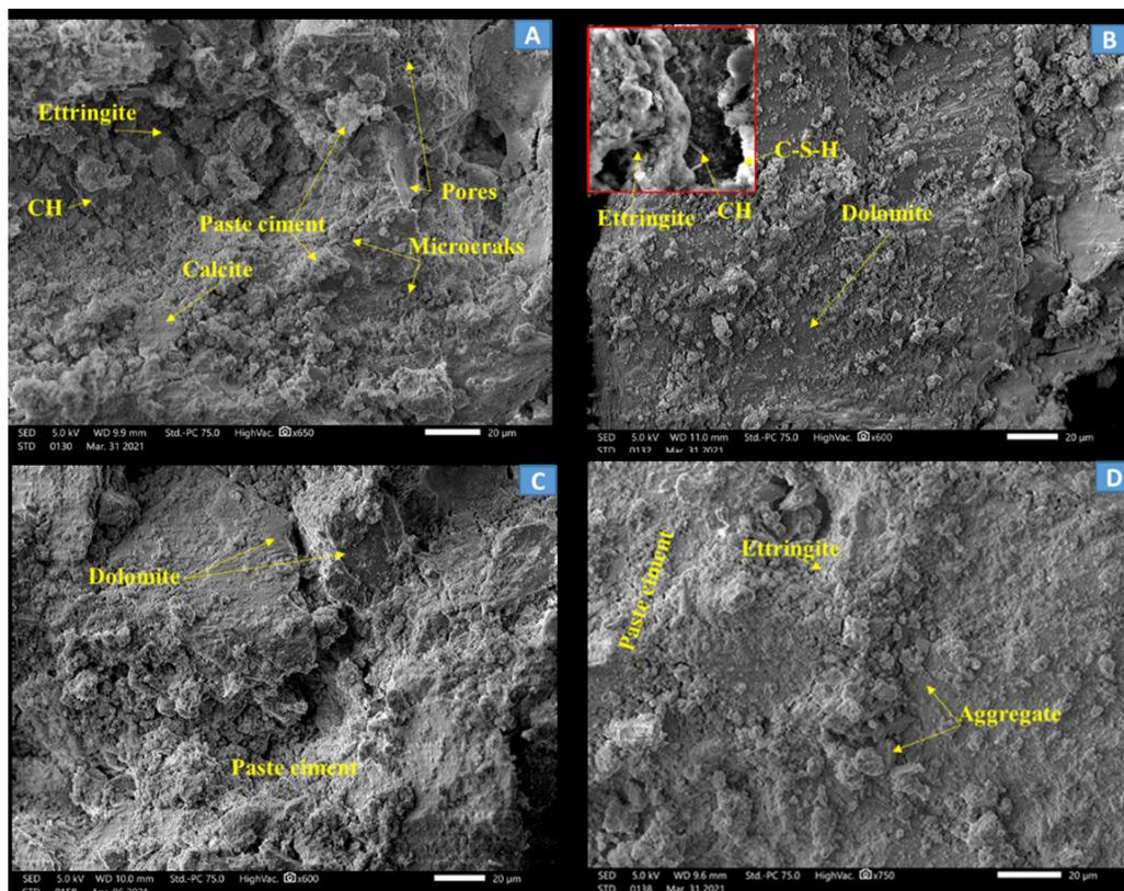
**Figure 12.** SEM images of mortar specimens. A: Quarry sand S1 ( $125 < \phi < 250 \mu\text{m}$ ); B: mining waste W1 ( $125 < \phi < 250 \mu\text{m}$ ); C: mining waste W4 ( $\phi < 2000 \mu\text{m}$ ); D: mining waste W2 ( $\phi < 125 \mu\text{m}$ )
