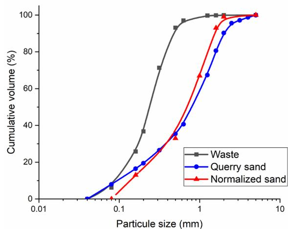
Figure 4. Particle size distribution of sand S4, standard sand and waste W4 ( $\phi < 2000 \mu\text{m}$ )
