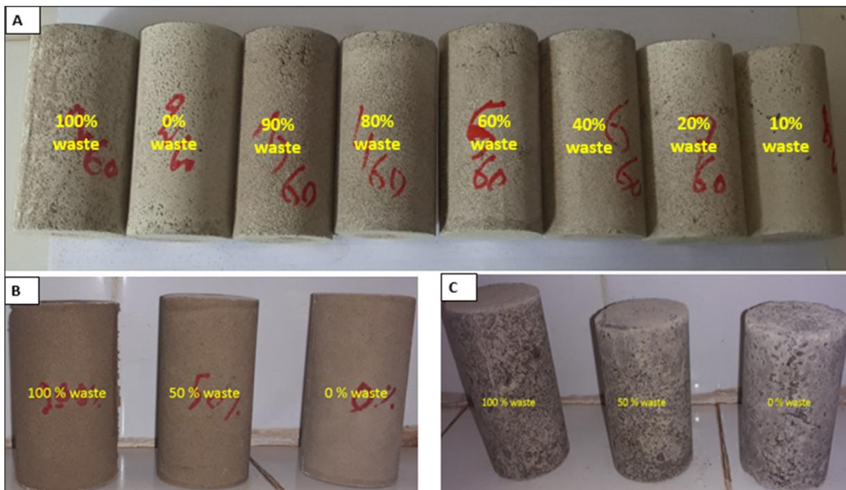
**Figure 3.** The appearance of prepared mortar specimens based on variable amounts of mining waste and quarry sand; (A) W1, S1 ( $125 < \phi < 250 \mu\text{m}$ ), (B) W2, S2 ( $\phi < 125 \mu\text{m}$ ) and (C) W3, S3 ( $250 \mu\text{m} < \phi$ )
