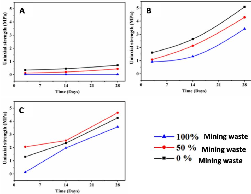
**Figure 10.** Compressive strength evolution in terms of curing time of mortar specimens based on mixtures A: W2, S2 ( $\phi < 125 \mu\text{m}$ ); B: W3, S3 ( $\phi > 250 \mu\text{m}$ ) and C: W4, S4 ( $\phi < 2000 \mu\text{m}$ )
