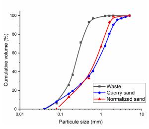
**Figure 4.** Particle size distribution of sand S4, standard sand and waste W4 ( $\phi < 2000 \ \mu m$ )
