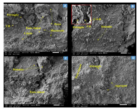
**Figure 12.** SEM images of mortar specimens. A: Quarry sand S1 ( $125 < \phi < 250 \ \mu m$ ); B: mining waste W1 ( $125 < \phi < 250 \ \mu m$ ); C: mining waste W4 ( $\phi < 2000 \ \mu m$ ); D: mining waste W2 ( $\phi < 125 \ \mu m$ )
