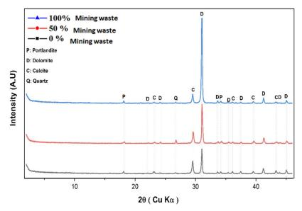
Figure 11. XRD spectra of cured mortar specimens of the mixtures W1, S1  $(125 < \phi < 250 \ \mu m)$  for 0, 40 and 100% of mining waste added
