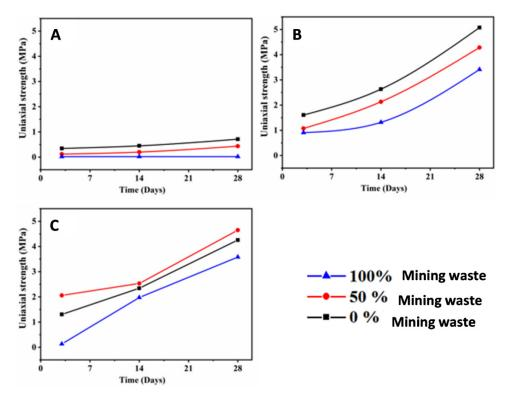
**Figure. 10.** Compressive strength evolution in terms of curing time of mortar specimens based on mixtures A: W2, S2 ( $\phi < 125 \mu$ m); B: W3, S3 ( $\phi > 250 \mu$ m) and C: W4, S4 ( $\phi < 2000 \mu$ m)
