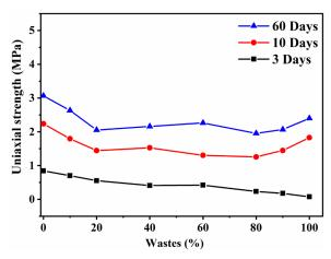
Fig. 9. Compressive strength of mortar specimens W1, S1 ( $125 < \phi < 250 \mu m$ ) at different percentage of waste cured for 3, 10 and 60 days
