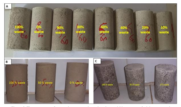
**Figure 3.** The appearance of prepared mortar specimens based on variable amounts of mining waste and quarry sand; (A) W1, S1 ( $125 < \phi < 250 \mu m$ ), (B) W2, S2 ( $\phi < 125 \mu m$ ) and (C) W3, S3 ( $250 \mu m < \phi$ )
