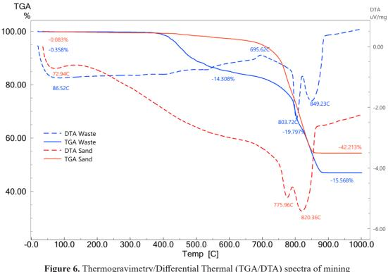
waste W4 ( $\phi < 2000 \ \mu m$ ) and finely quarry sand S4 ( $\phi < 2000 \ \mu m$ )
