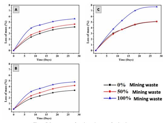
Figure 7. Loss on mass of specimens in terms of curing time. (A) W4, S4 ( $\phi < 2000 \ \mu m$ ), (B) W3, S3 ( $\phi > 250 \ \mu m$ ), (C) W2, S2 ( $\phi < 125 \ \mu m$ )
