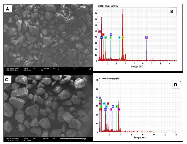
**Figure 8.** SEM images of (A) W0, CMT mining waste and (C) W4, OMC mining waste. EDX spectra of (B) W0, CMT washed mining waste and (D) W4, OMC rewashed mining waste ( $\phi < 2000 \ \mu m$ )
