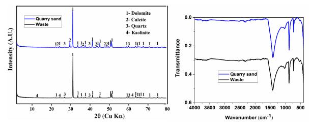
Figure 5. XRD and FTIR spectra of sand S4 and mining waste W4 ( $\phi$ < 2000 µm)
