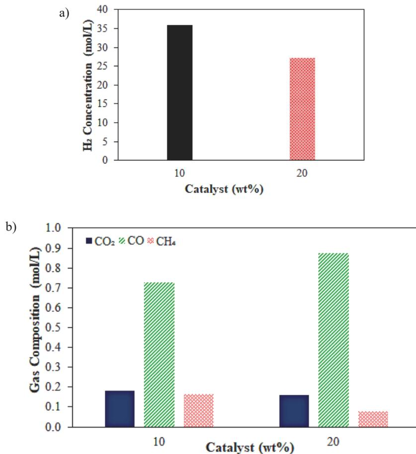
Figure 4. Effect of catalyst addition on syngas composition: a) H<sub>2</sub> concentration, b) Other gasses
