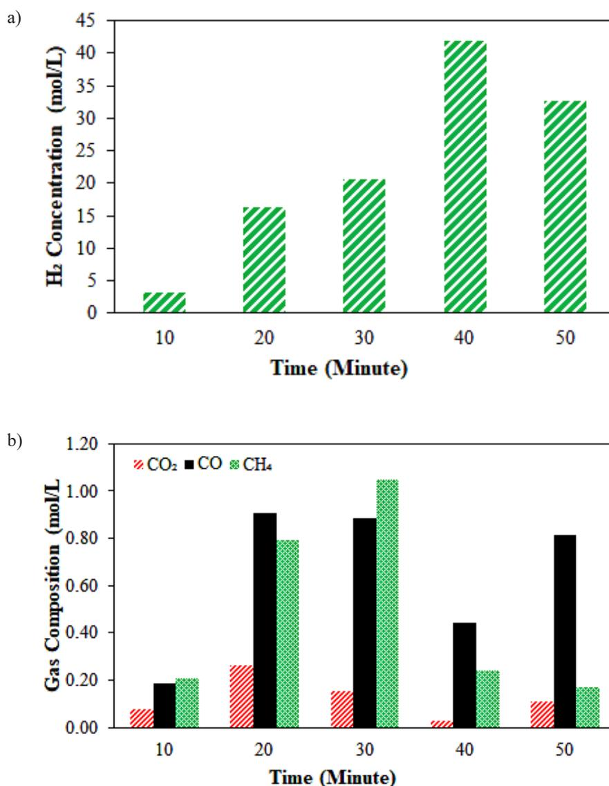
Figure 2. Syngas composition with reaction time variation: a) H<sub>2</sub> concentration, b) Other gasses
