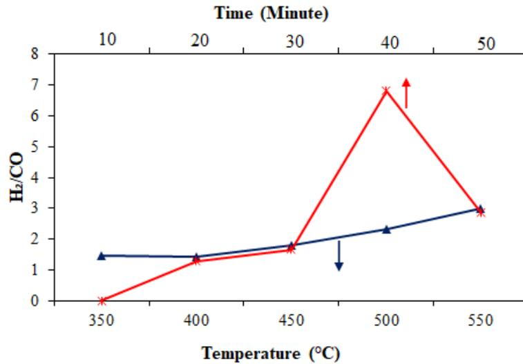
Figure 3. Effect of gasification temperature and time on H<sub>2</sub>/CO ratio syngas
