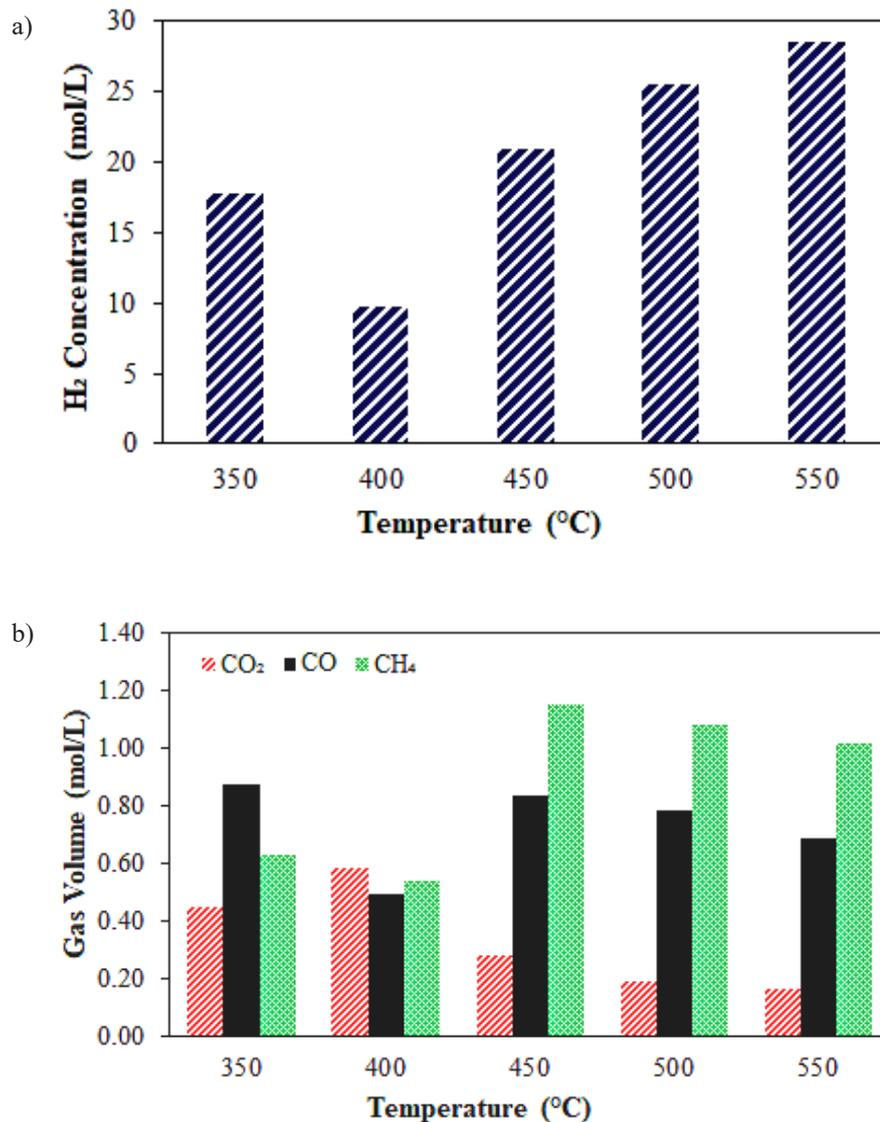
**Figure 1.** Syngas composition with temperature variation (a) H<sub>2</sub> concentration; (b) Other gases
