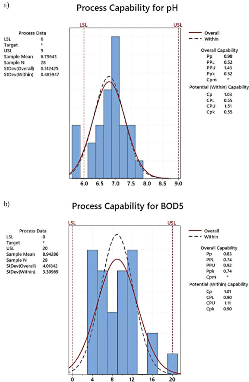
Fig. 3. Process capability for the assessed parameters
