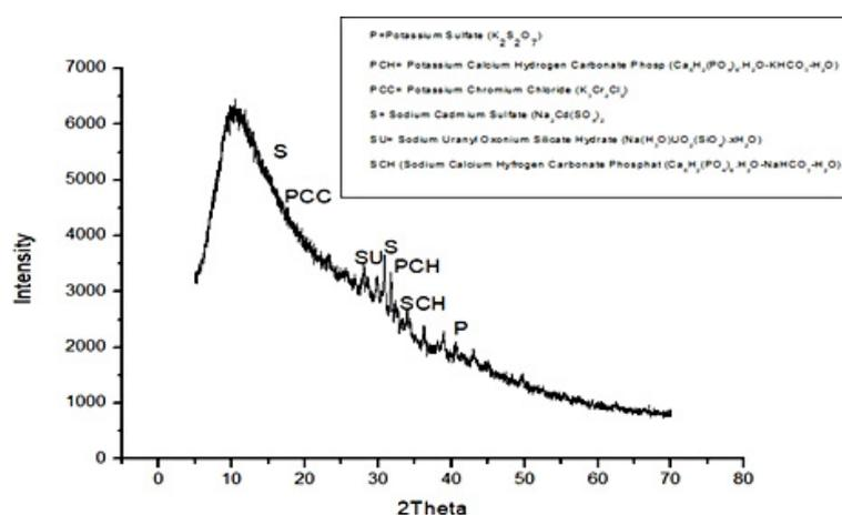
Figure 4. Results of XRD analysis of catalyst
