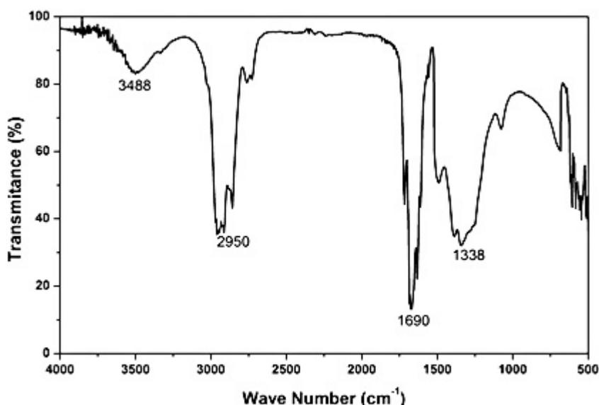
**Figure 3.** Results of FTIR analysis of catalyst
