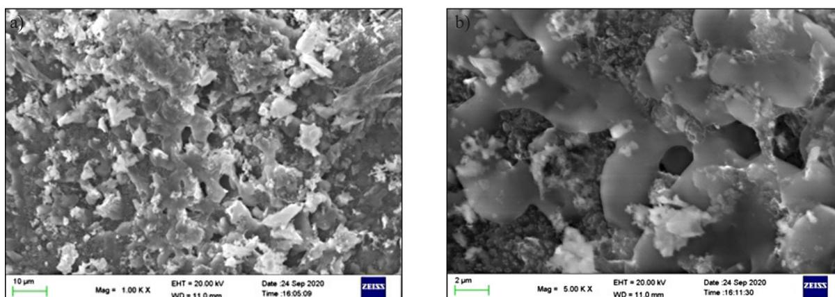
Figure 5. SEM of catalyst with magnification (a) 1000× (b) 5000×
