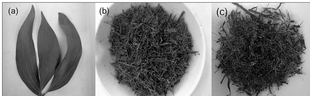
**Figure 1.** AcLW biomass samples; (a) Acacia leave, (b) shredded AcLW, and (c) alkaline pretreated AcLW
