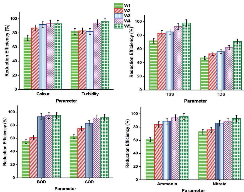
Figure 3. The removal of physicochemical parameters from landfill leachates
