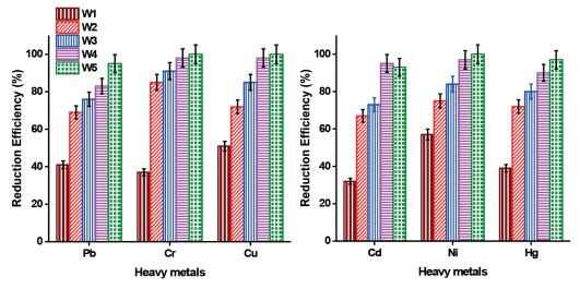
Figure 1. The removal of heavy metals from landfill leachates
