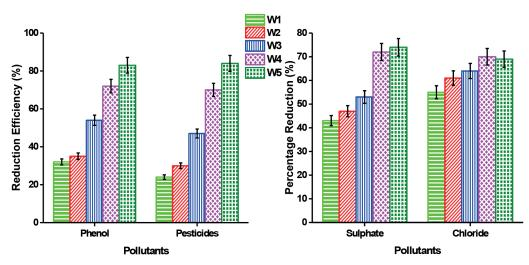
Figure 2. The removal of phenol, pesticides, sulphate and chlorides from landfill leachates
