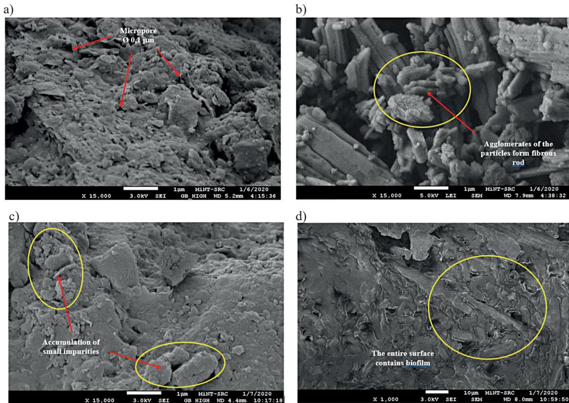
**Figure 4.** SEM micrographs of media before (a–b) and after (c–d) ripening. a) and c) river sand media. b) and d) *A. granosa* shell media
