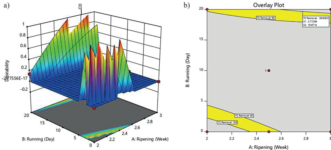
**Figure 3.** (a) 3D desirability graph and (b) overlay plot of the best operating parameters of slow sand filter with a combination media of river sand and *Anadara granosa* shell in removing coliforms
