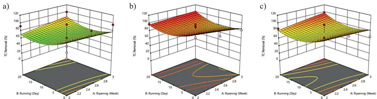
**Figure 2.** 3D response surface plot for total coliform removal efficiency by using slow sand filter with (a) river sand, (b) combination, and (c) *A. granosa* shell
