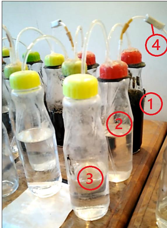
**Figure 1.** BMP tests reactors. 1 – digester, 2 – water container, 3 – displaced water container, 4 – biogas control valve
