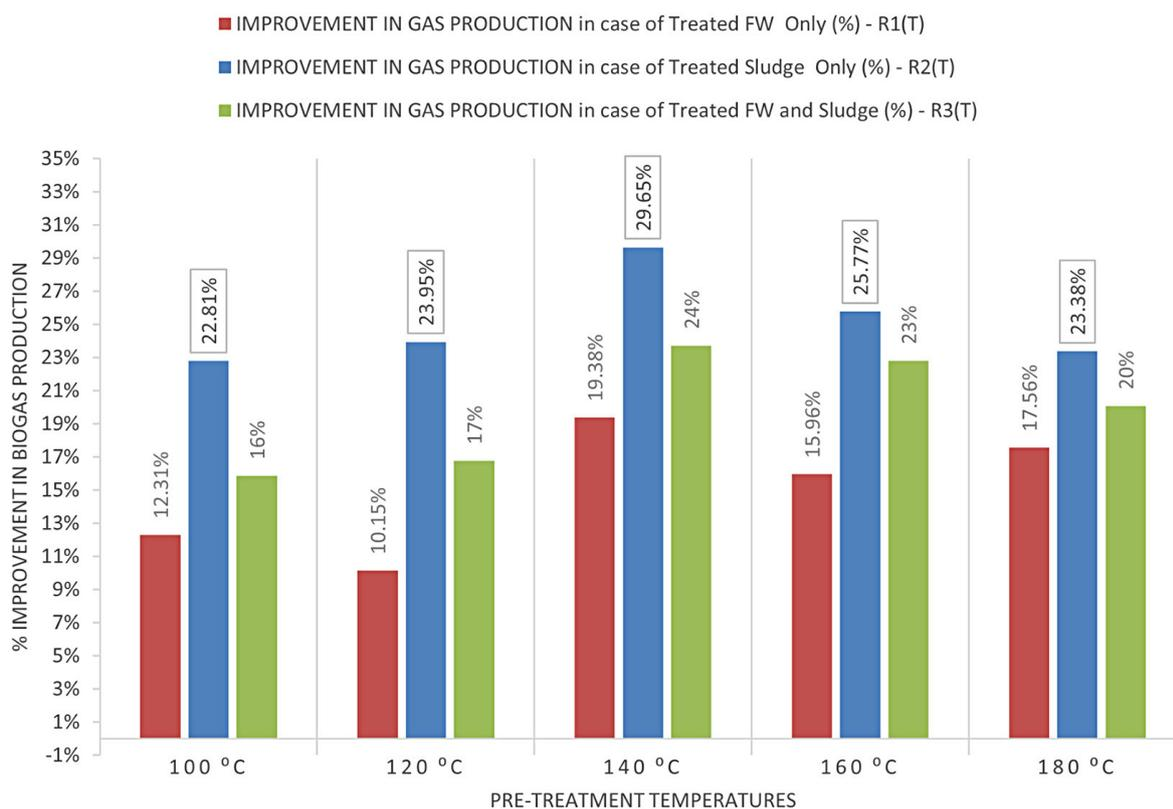
**Figure 7.** Improvement in biogas production (%)
