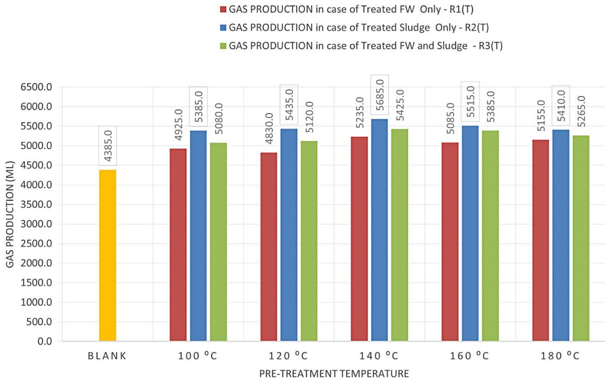
Figure 6. Biogas production in various pre-treatment temperatures and blank
