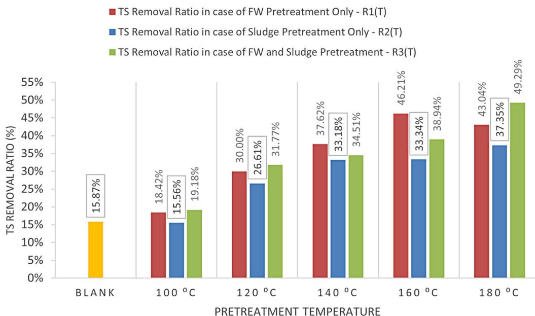
Figure 3. Total solids removal ratio
