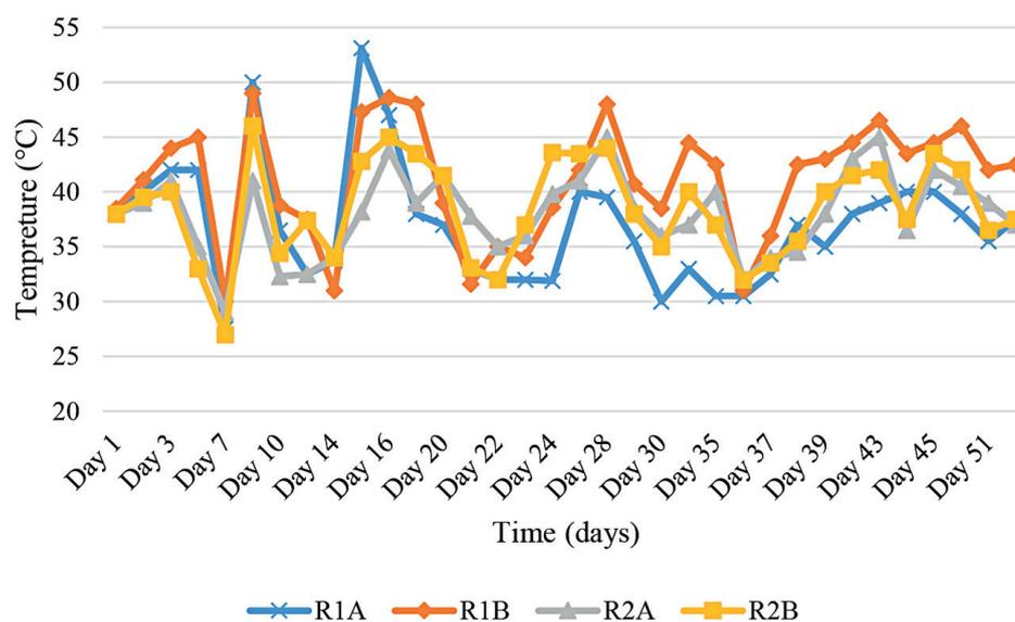
Figure 2. Temperature profile during the composting period
