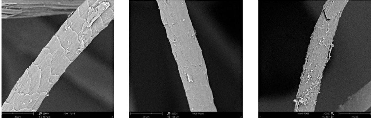
**Figure 3.** SEM microphotographs: X – reference wool sample used for the experiment, A – wool sample from the bottom of the pot, B – sample of wool mixed with the crop substrate
