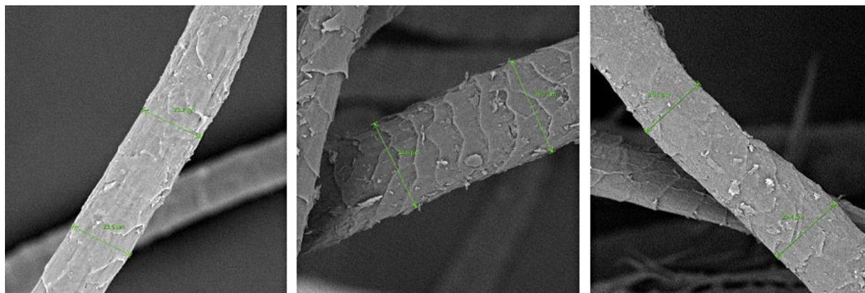
**Figure 5.** Example of the application of Fiber Metric software to determine the thickness of the fibers
