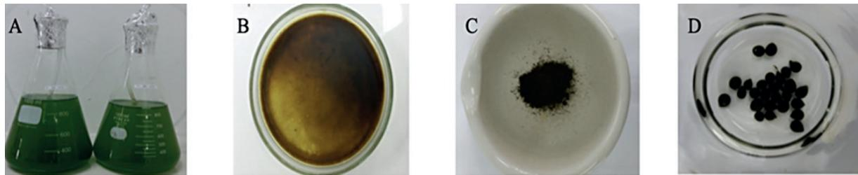
**Figure 1.** Biosorbent preparation (A) *Chlorella* sp.; culture (B) dried *Chlorella* sp.; (C) *Chlorella* sp powder; (D) immobile *Chlorella* sp. (microalgae beads as biosorbent)
