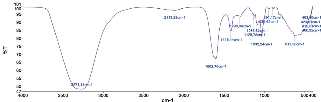
Figure 5. Mixed microalgae biosorbent ftir analysis result after the biosorption process
