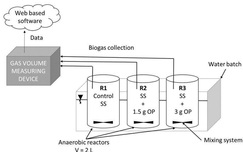
**Figure 1.** The scheme of operational set-up
