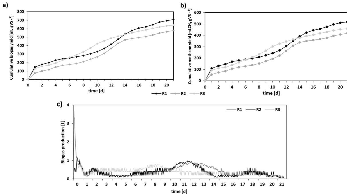
**Figure 3.** Cumulative biogas (a) and methane (b) yields as well as daily biogas production (c)
