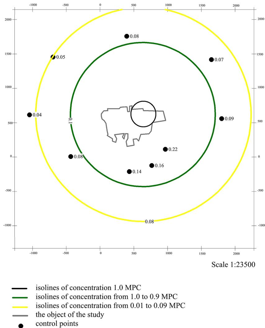
Fig. 6. Map of the concentration fields of methanol (methyl alcohol) in the air pool
