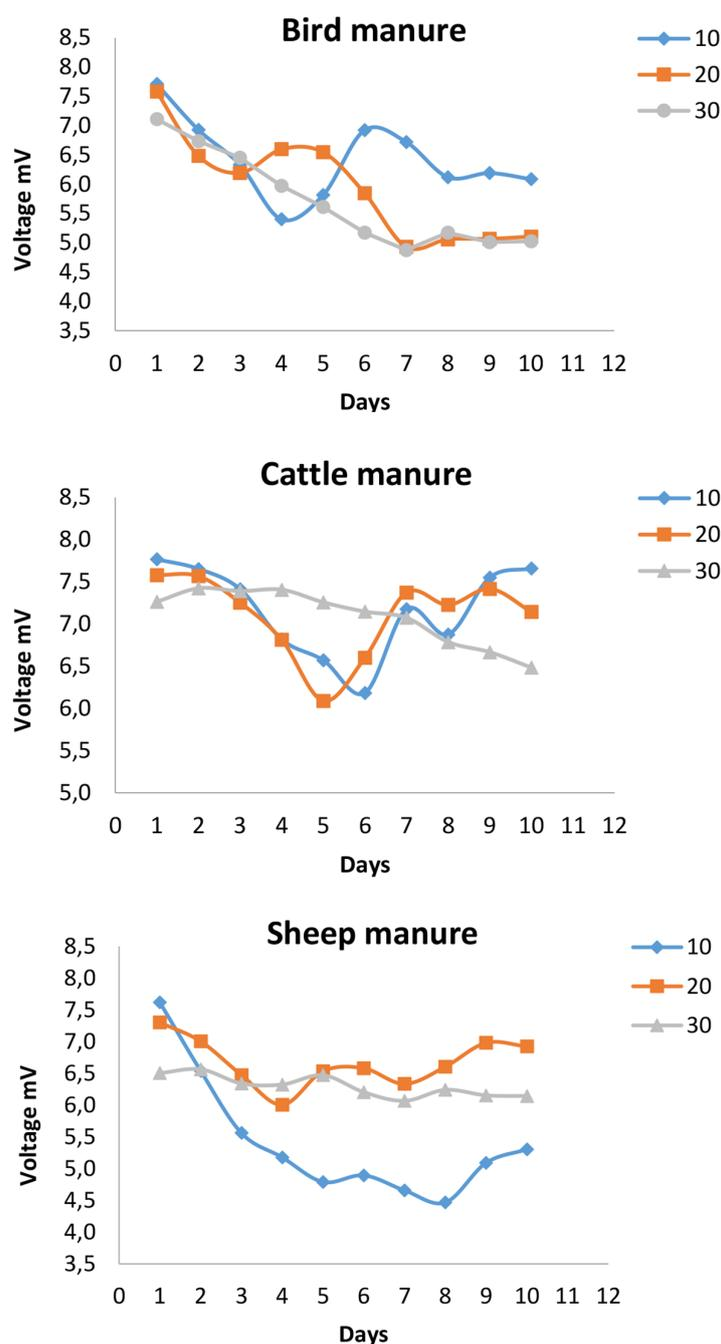
Figure 2. Voltage generated by varying amounts of different types of manure (thick wire)
