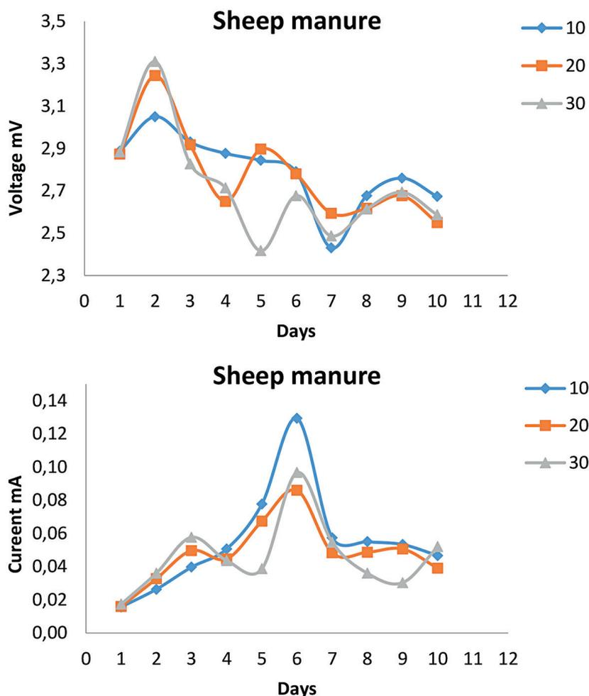
Figure 4. Voltage and current generated by varying amounts of different types of manure (thin wire)
