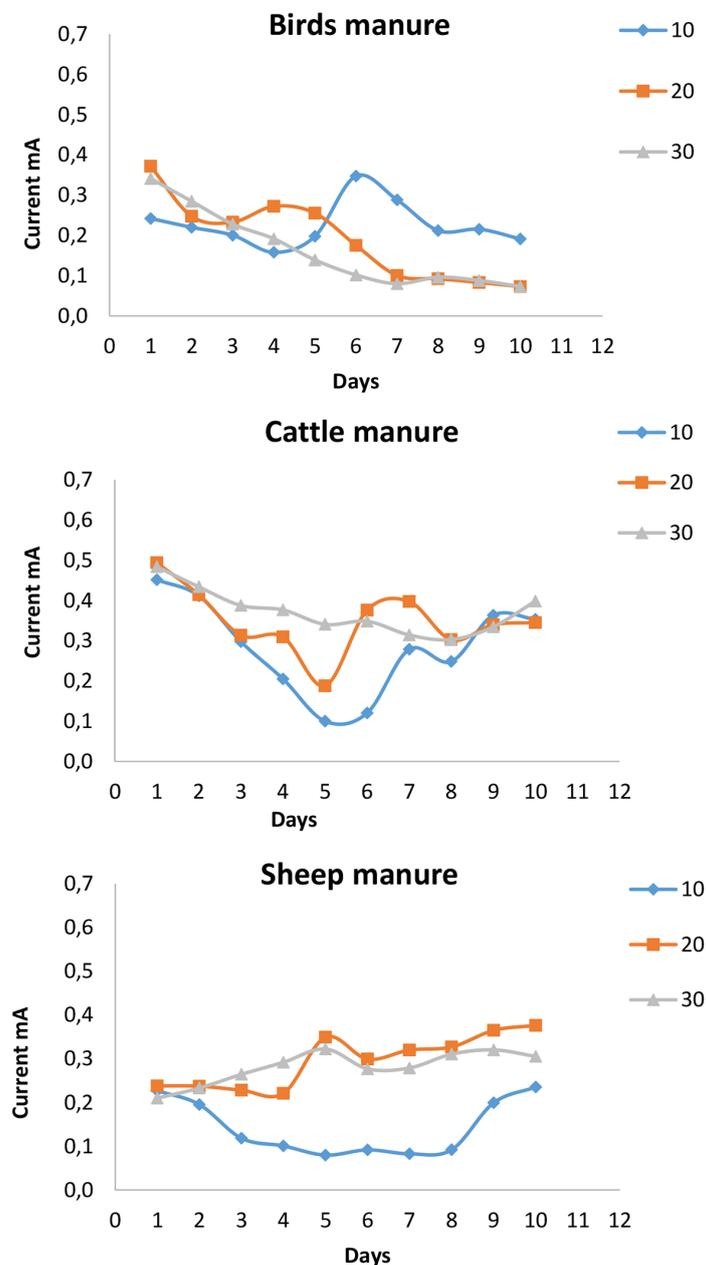
Figure 3. Current generated by varying amounts of different types of manure (thick wire)
