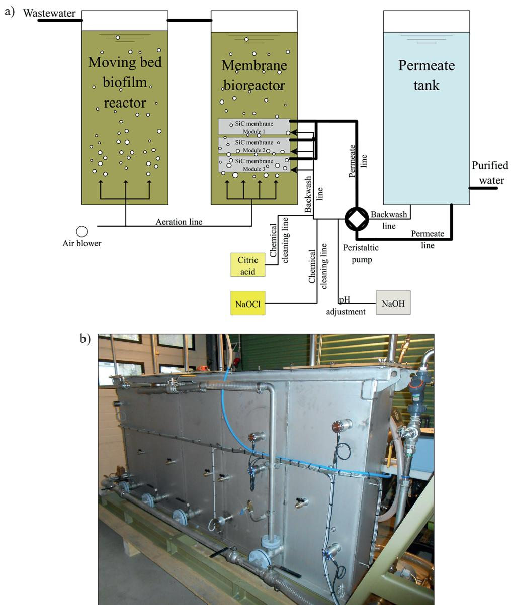
**Figure 1.** Schematic of ceramic MBR & MBBR pilot plant in Ås, Norway (Dzihora, 2021)
