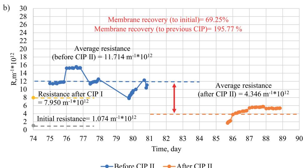
**Figure 4.** Cleaning efficiency for CIP I & CIP II
