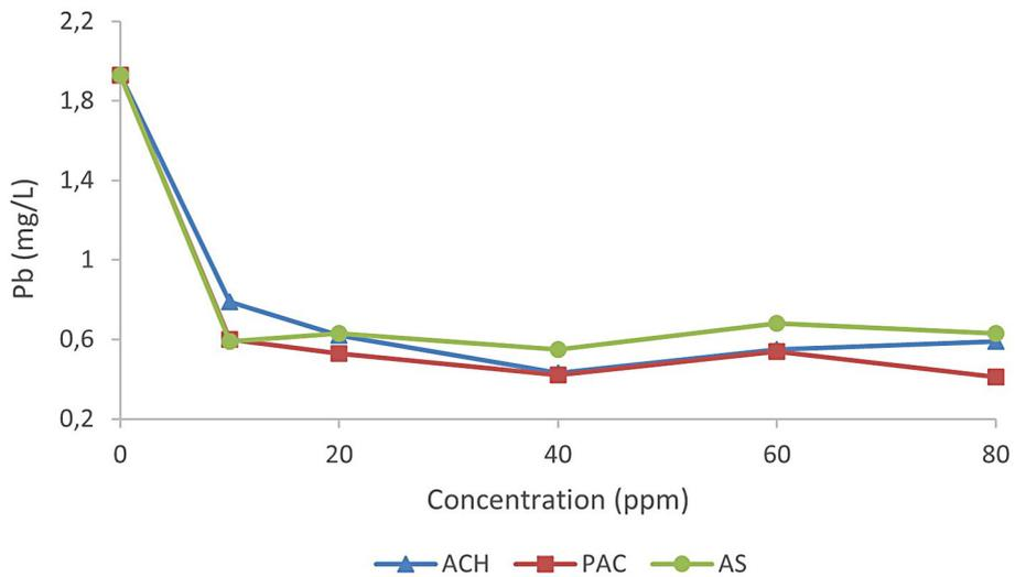
**Figure 6.** Effect of coagulant concentration on Pb reduction
