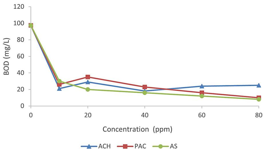
Figure 3. Effect of coagulant concentration on BOD reduction
