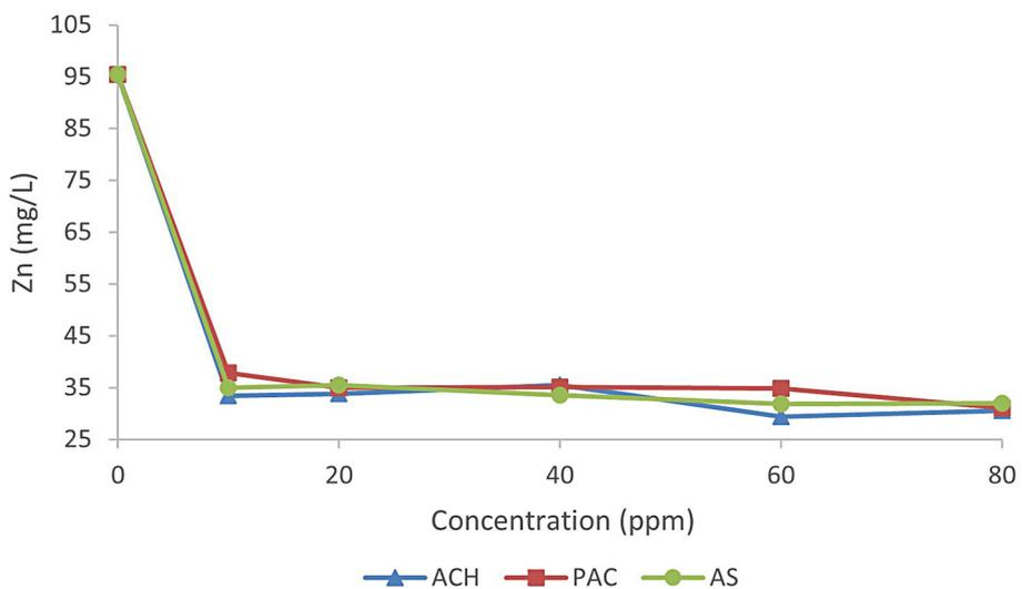
**Figure 7.** Effect of coagulant concentration on Zn reduction
