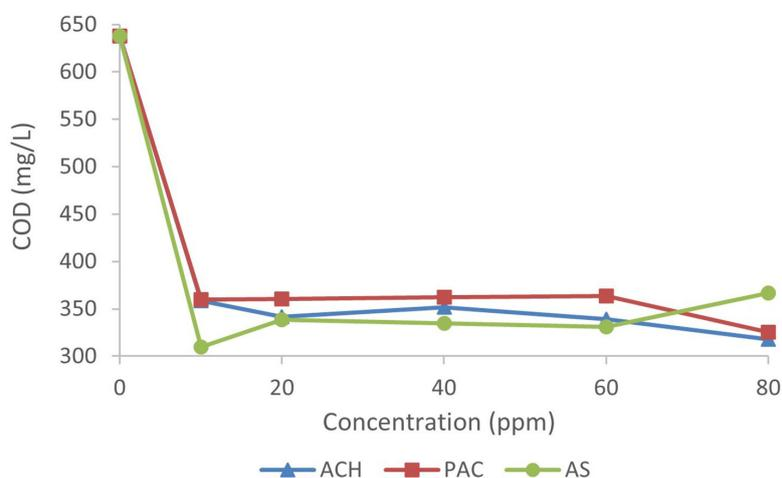
Figure 2. Effect of coagulant concentration on COD reduction
