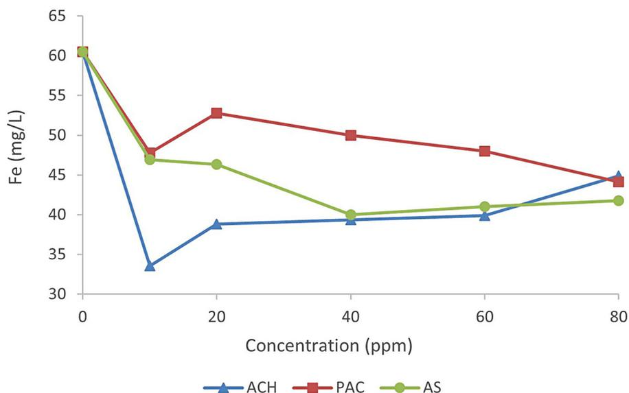
Figure 8. Effect of coagulant concentration on Fe reduction
