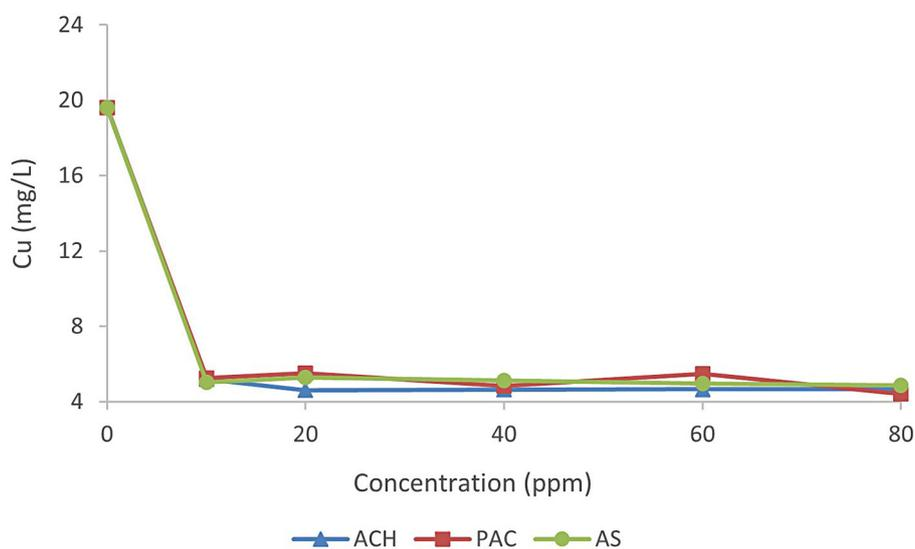
Figure 4. Effect of coagulant concentration on Cu reduction
