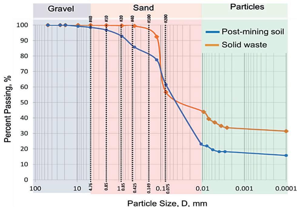
**Figure 3.** Analysis of post-mining soil and solid waste grain-size distribution curve
