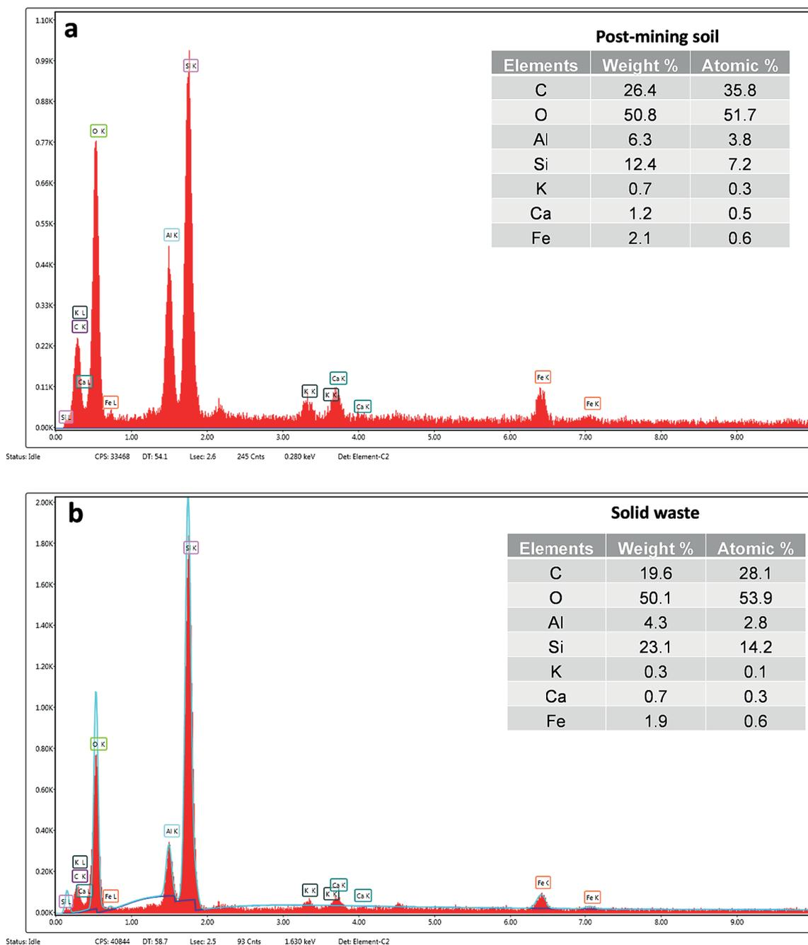
**Figure 7.** EDX spectrum of both samples; post-mining soil (a) and solid waste (b)
