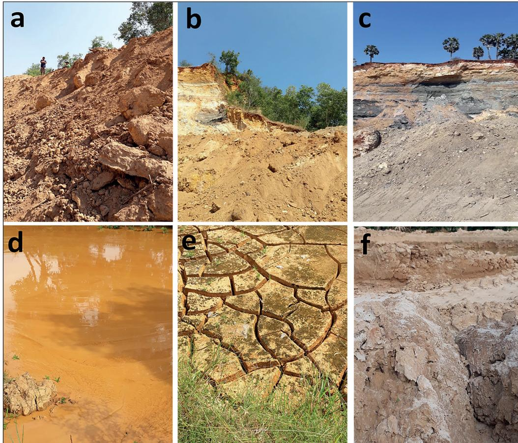
**Figure 2.** Typical samples: (a, b, c) the post-mining soil and (d, e, f) solid waste from silica sand purification
