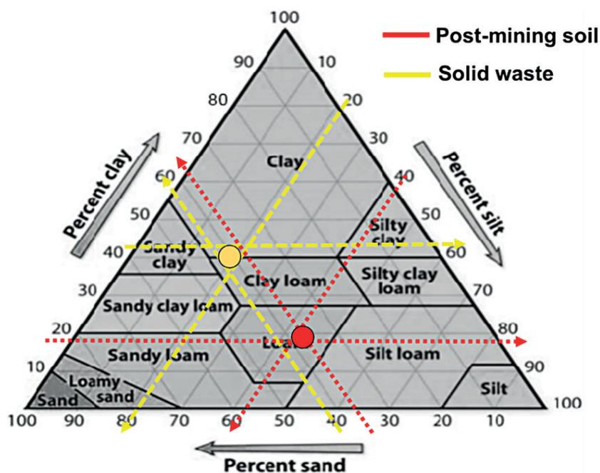
Figure 4. Characteristics of post-mining soil and solid waste in soil texture triangle
