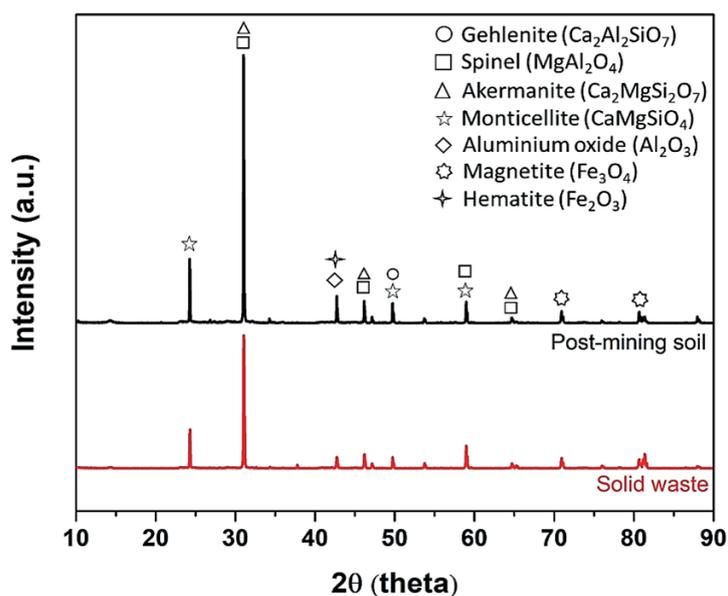
Figure 5. XRD pattern of samples (post-mining soil and solid waste)
