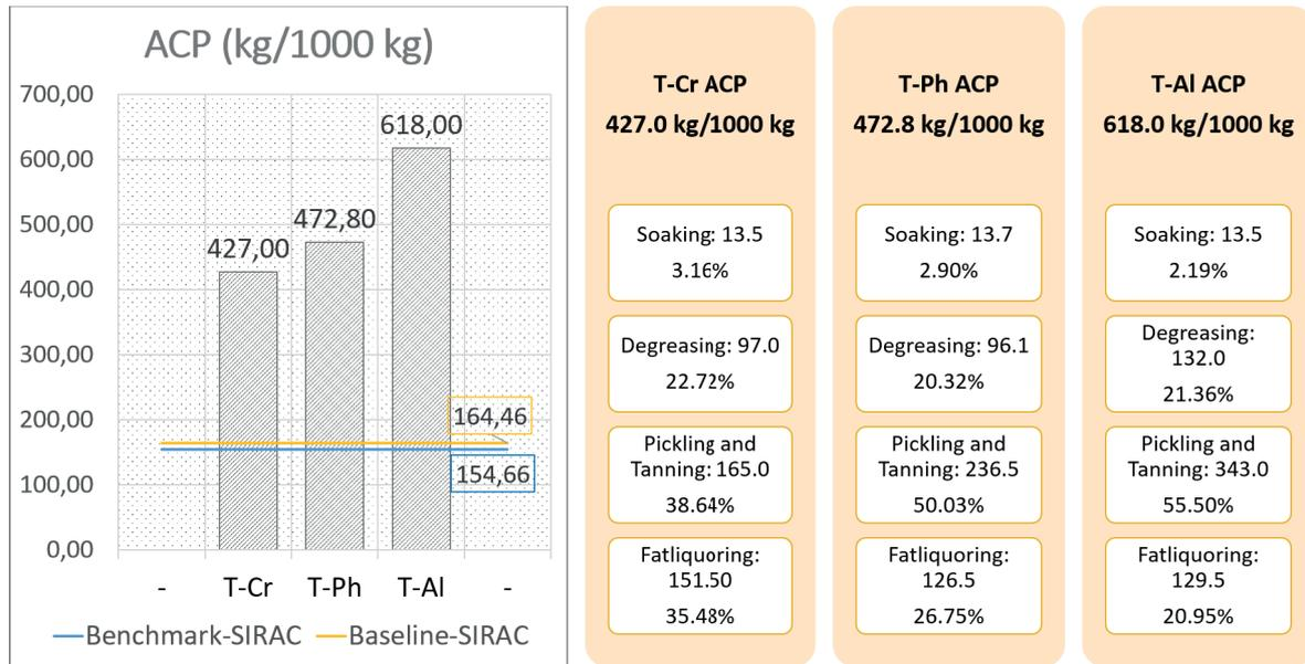
**Figure 3.** Comparison of the indicator amount of chemicals used per initial processed leather from tanning techniques and percentage per operation
