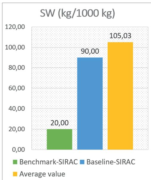
**Figure 5.** Value of the indicator of the amount of waste generated by the initial leather processed from the tanning techniques
