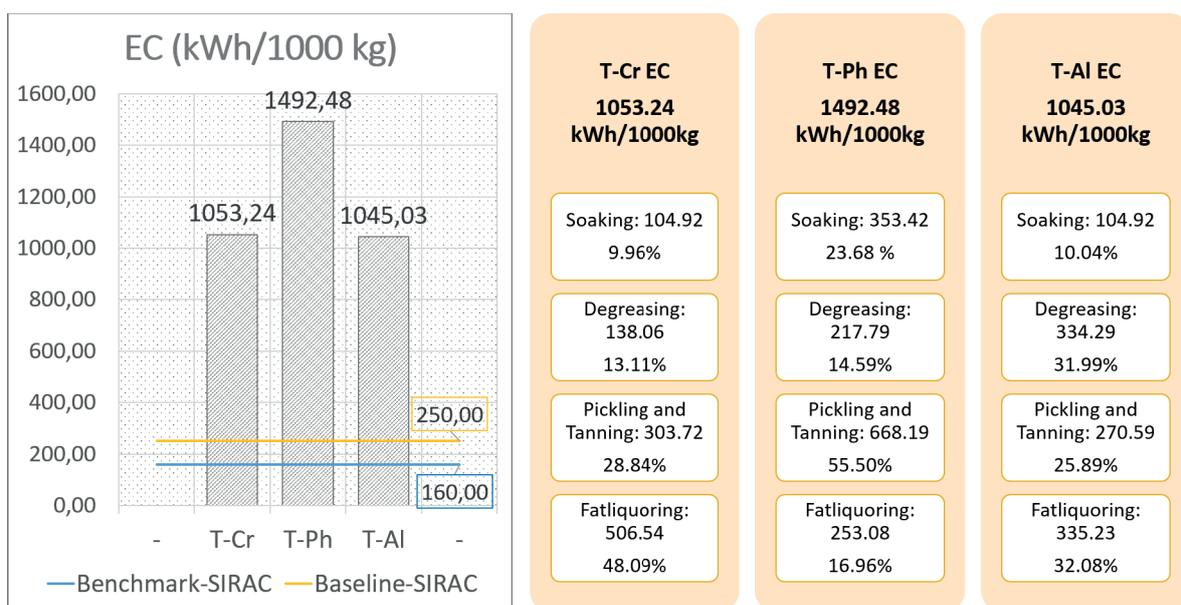
**Figure 4.** Comparison of the indicator energy consumption by initial processed leather of the tanning techniques and percentage per operation
