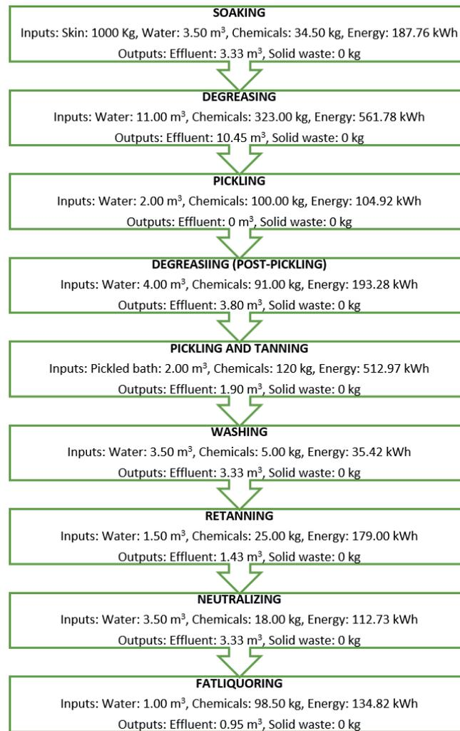
Figure 7. Inputs and outputs of the T-OPh
