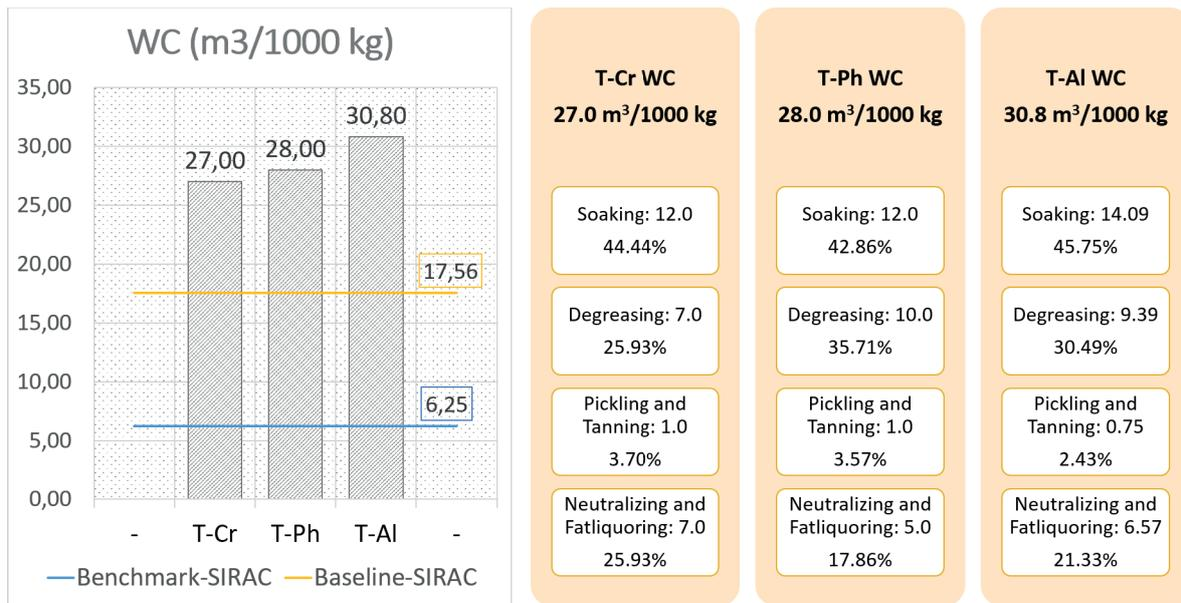
**Figure 2.** Comparison of water consumption per initial processed leather of tanning techniques and percentage per operation
