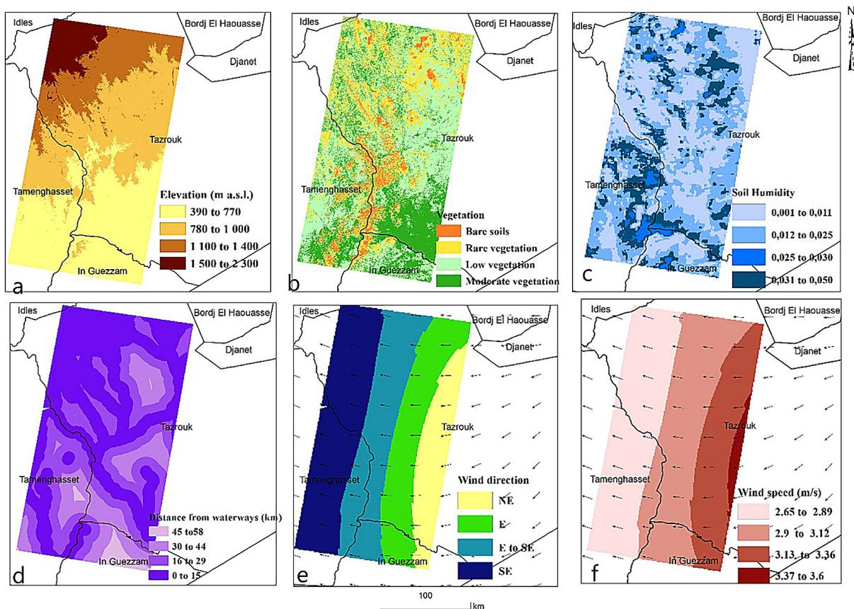
Figure 2. Factors maps: a) elevation map; b) vegetation map; c) soil moisture map; d) distance from waterways; e) wind direction; f) wind speed
