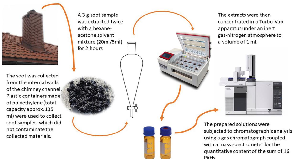
**Figure 2.** Scheme for soot sampling and preparation
