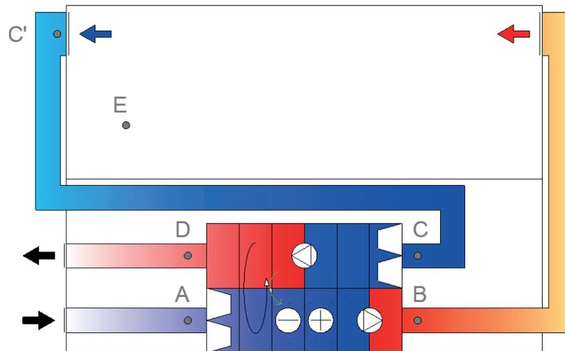
**Figure 1.** Locations of air cleaning devices (A, B, C, C', D, E).
