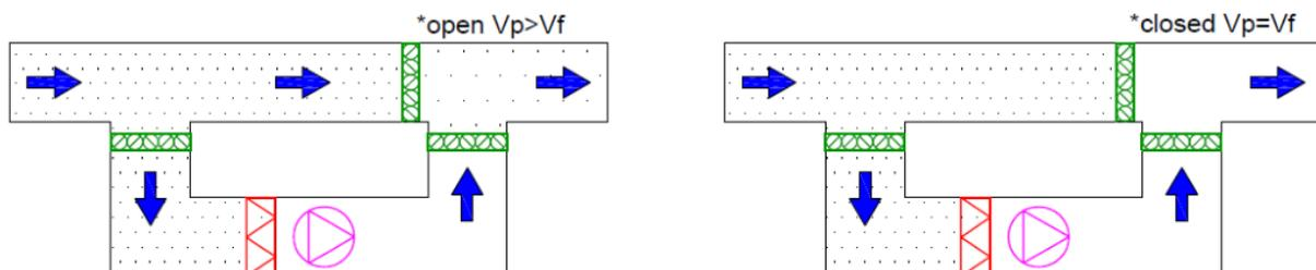
**Figure 2.** The idea of a cleaning device in the by-pass duct, based on [3a]
