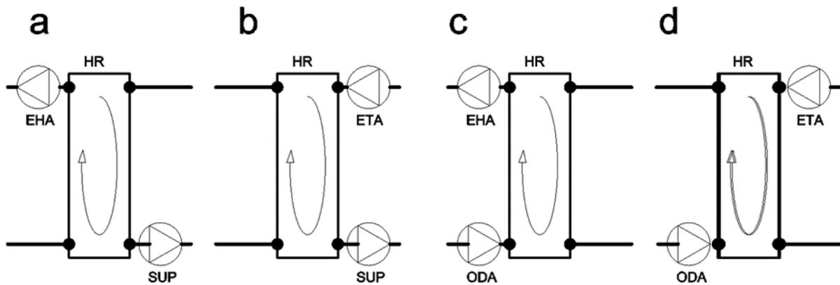
**Figure 4.** Possible configurations of the fans in relation to the heat recovery system in the air handling unit
