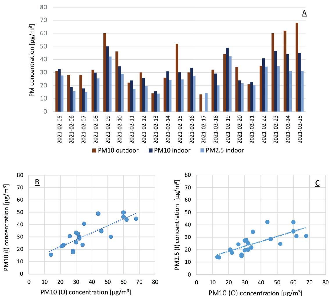
**Figure 4.** a) Relationship between 24-h average  $PM_{10}$  and  $PM_{2.5}$  concentrations measured in indoor air and  $PM_{10}$  measured in outdoor air for the period 5.02.2021–25.02.2021; b) Correlation between the 24-h average  $PM_{10}$  (I) indoor and  $PM_{10}$  (O) outdoor concentrations measured at the monitoring network station and c) correlation between the 24-h average  $PM_{10}$  (I) indoor and  $PM_{2.5}$  (O) concentrations measured at the monitoring network station
