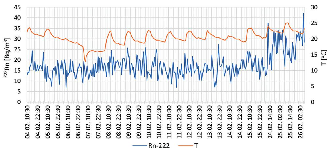
**Figure 5.** Changes in indoor air temperature and  $^{222}\text{Rn}$  activity concentration in the air inside the study room during the period 5.02–25.02
