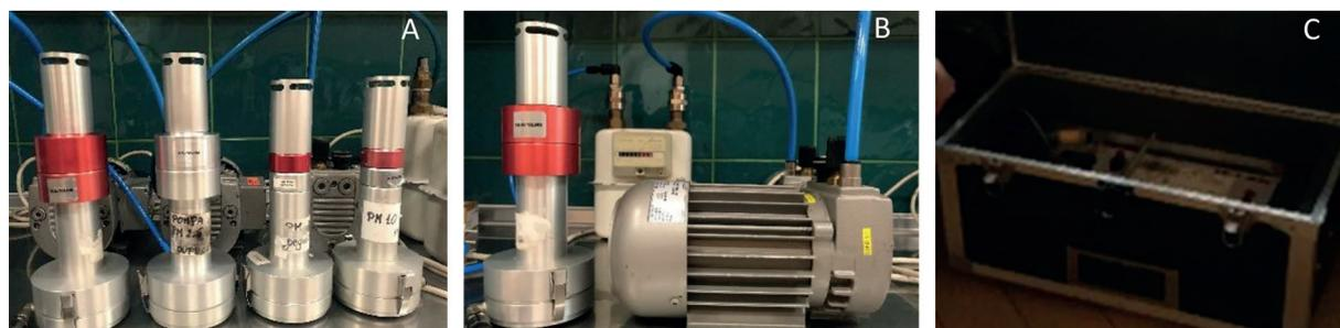
**Figure 2.** Particulate measuring devices in outdoor and indoor air used for the study at the spa; a) Harvard impactor for measurement of  $\text{PM}_1$ ,  $\text{PM}_{2.5}$ ,  $\text{PM}_{10}$  and fractions, b) Measurement set: impactor, Becker pump, ACTARIS G2.5 GALLUS 2000 gas meter; c) Vacuum pump – Air Diagnostics and Engineering, Air sampling pump, model SP-280E
