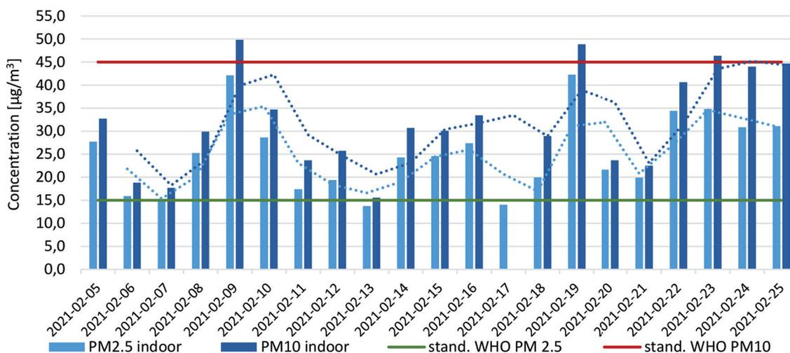
**Figure 3.** The average 24-h concentrations of PM<sub>10</sub> and PM<sub>2.5</sub> measured in the period of 5.02.2021–25.02.2021 in indoor air
