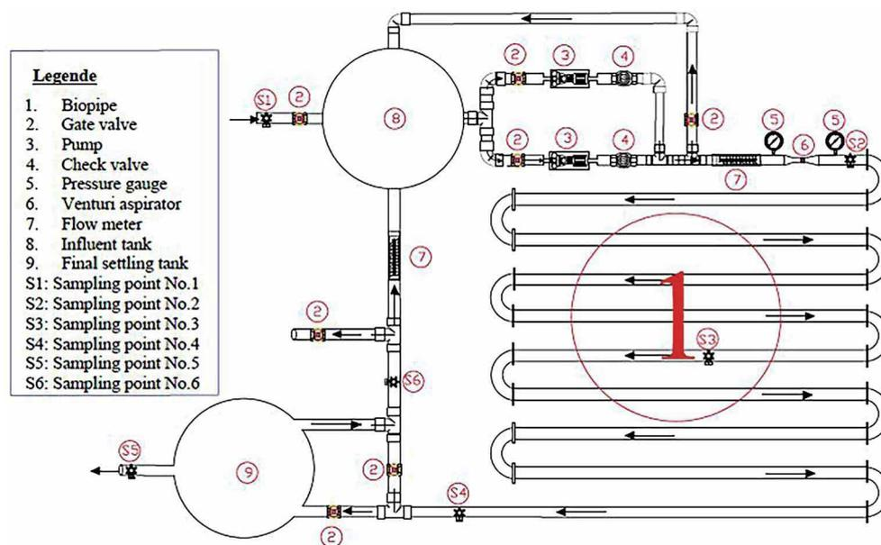
Figure 1. Schematic diagram of Biopipe system pilot plant
