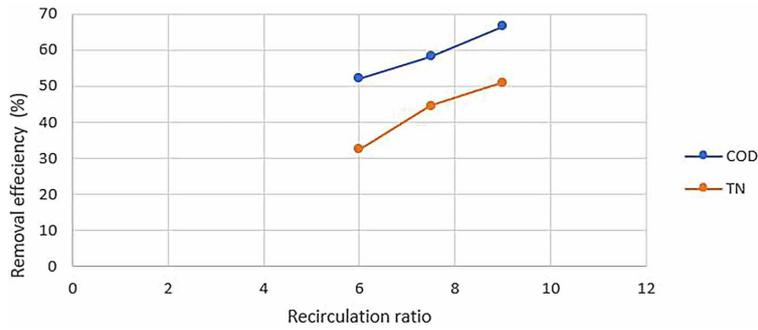
**Figure 9.** Effect of recirculation ratio on COD and TN removal efficiencies
