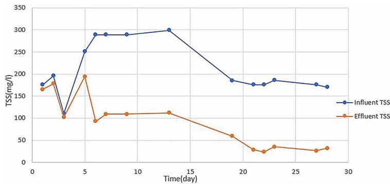
Figure 7. Temporal variation of influent and effluent TSS values during the startup period
