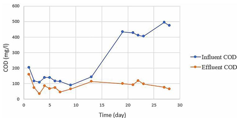
Figure 5. Temporal variation of influent and effluent COD values during the startup period
