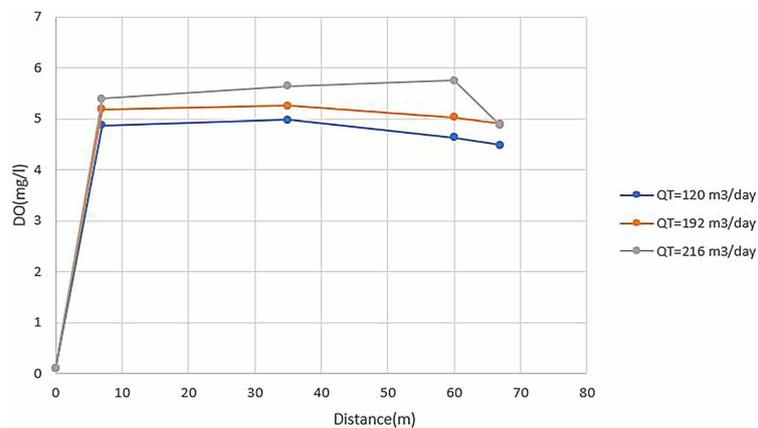
**Figure 11.** Longitudinal distribution of DO concentration
