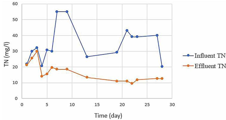
Figure 6. Temporal variation of influent and effluent TN values during the startup period
