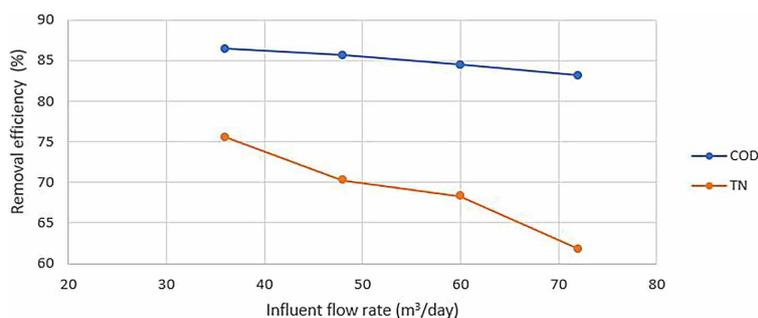
Figure 8. Effect of influent flowrate on COD and TN removal efficiencies
