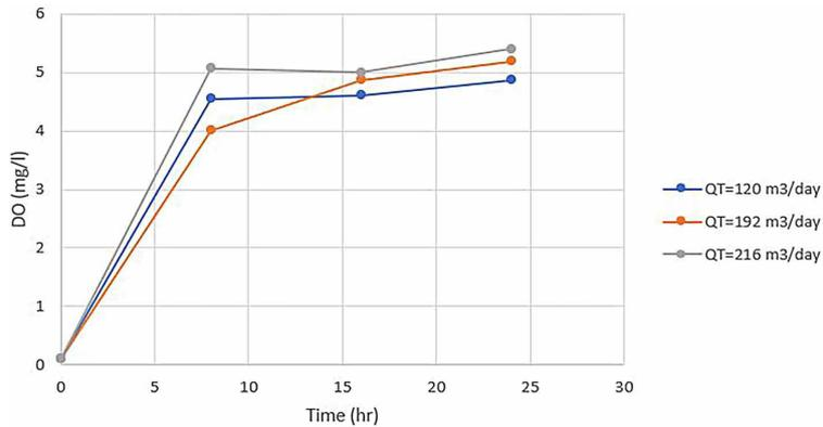
**Figure 10.** Temporal variation of DO concentration at different total flow rate
