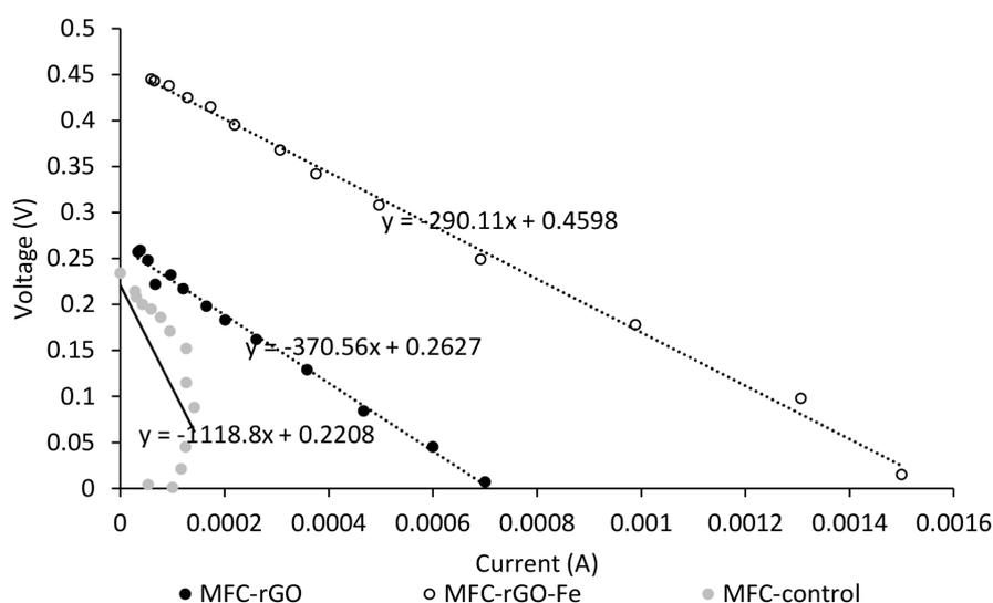
Figure 5. Polarization curves for all tested MFCs
