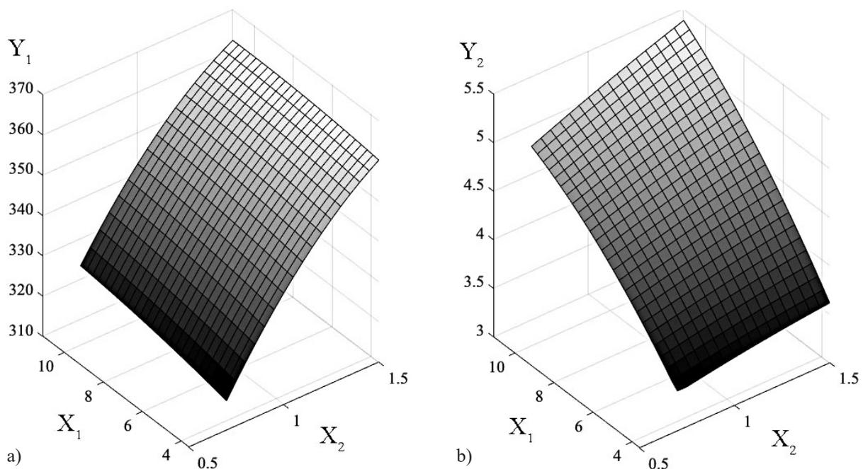
**Figure 1.** 3D surface predictions of cardboard properties using KROHUR: absolute resistance to compression (a) and compressive strength in the transverse direction (b)
