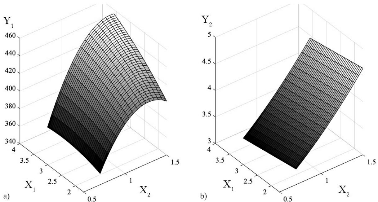
**Figure 3.** 3D surface predictions of cardboard properties using KROHAM: absolute resistance to compression (a) and compressive strength in the transverse direction (b)
