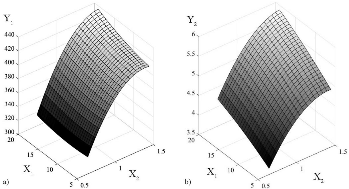
**Figure 2.** 3D surface predictions of cardboard properties using KROHMEL: absolute resistance to compression (a) and compressive strength in the transverse direction (b)
