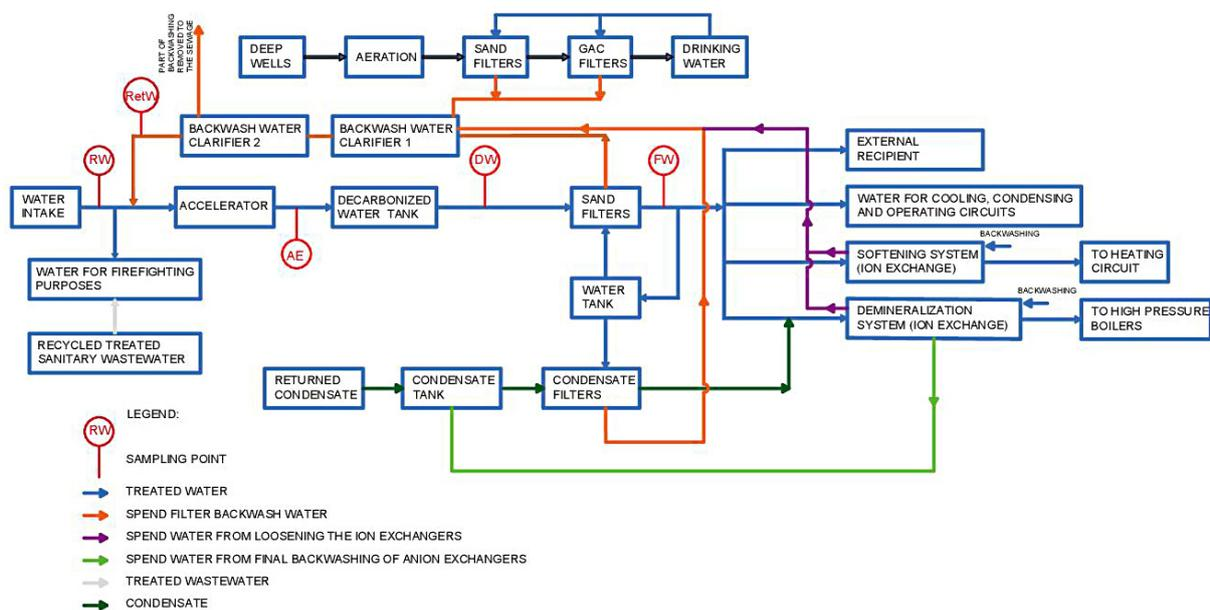
Fig. 1. Scheme of the WTP with recycled water streams and water sampling points
