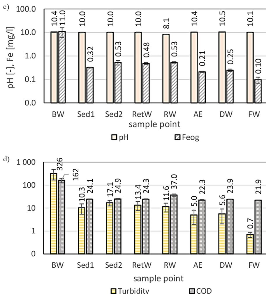
**Fig. 2. Cont.** Changes in the quality of water and recycled backwashings during treatment a) conductivity; b) hardness and alkalinity; c) pH and iron concentration; d) COD and turbidity
