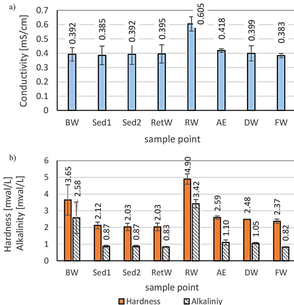
Fig. 2. Changes in the quality of water and recycled backwashings during treatment a) conductivity; b) hardness and alkalinity; c) pH and iron concentration; d) COD and turbidity
