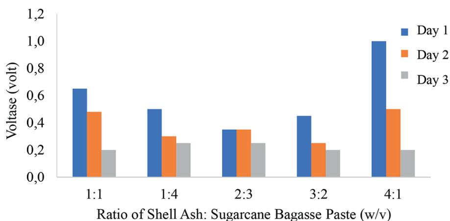
Figure 5. Bioelectrolyte voltage measurement results
