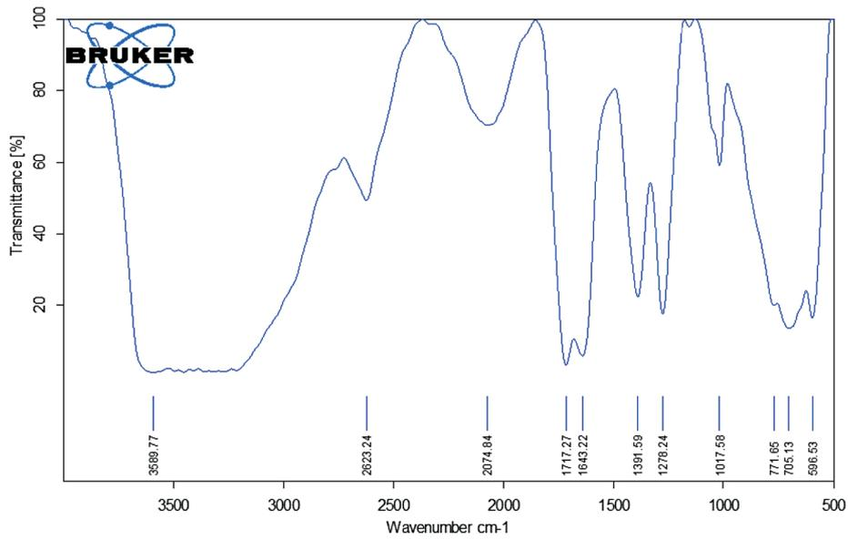
Figure 3. FTIR spectrum of hydrolysis products
