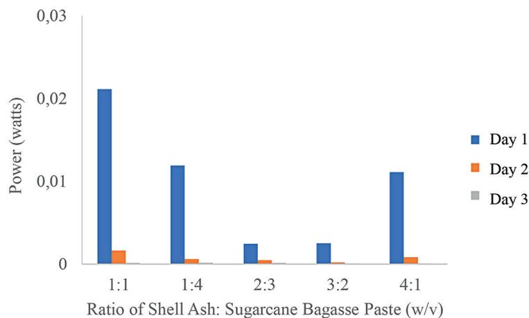
Figure 7. Bioelectrolyte power measurement results
