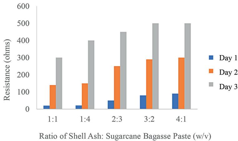
Figure 6. Results of measurement of bioelectrolyte barriers
