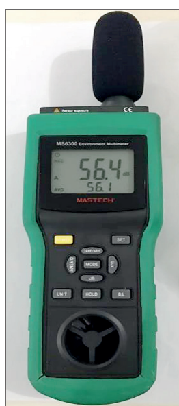
Figure 4. Noise level measurement using a sound meter
