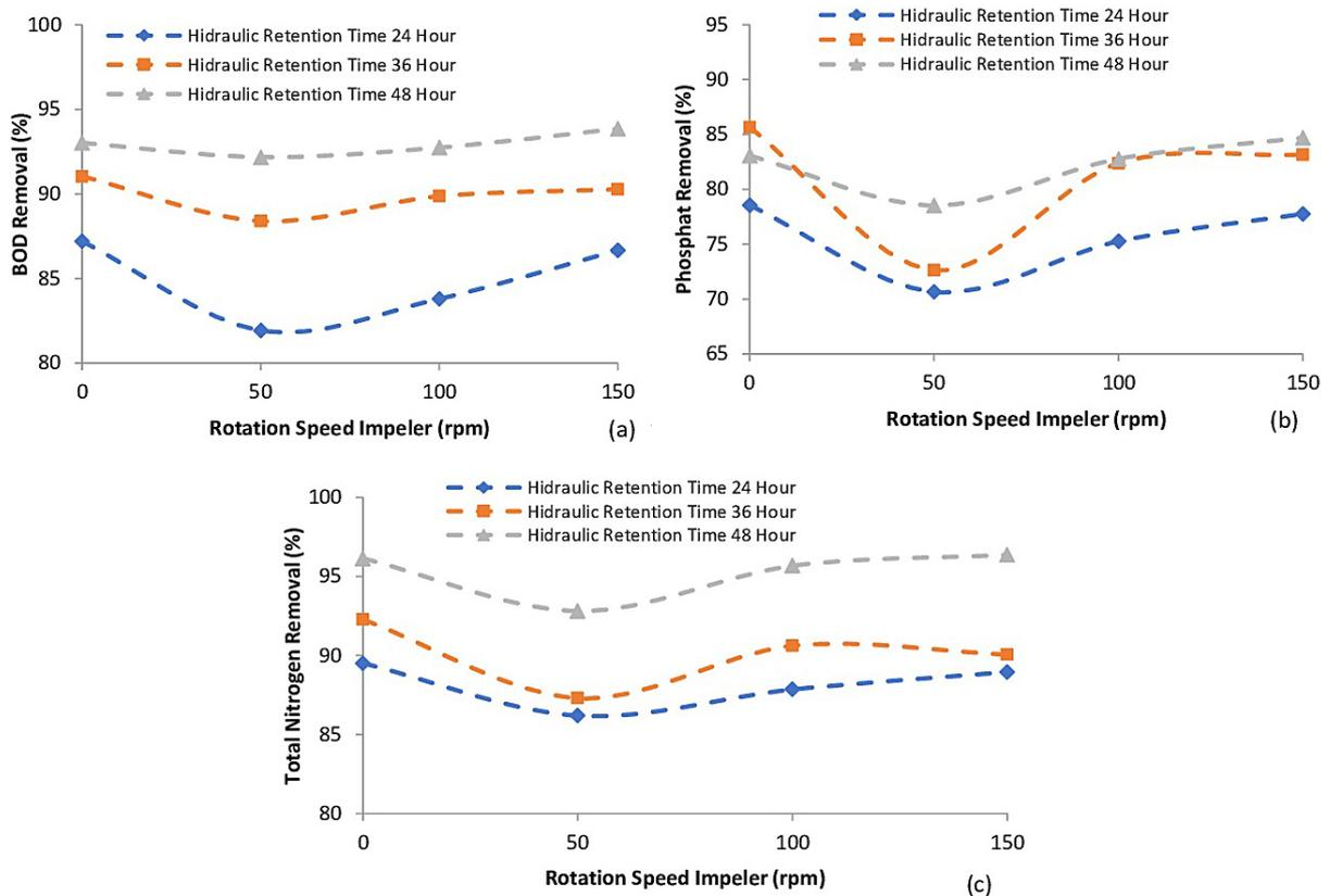
**Figure 2.** The decrease in (a) BOD<sub>5</sub>, (b) phosphate, and (c) total nitrogen in the sequencing batch reactor in terms of hydraulic retention time
