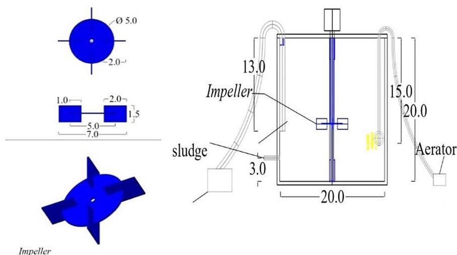
Figure 1. Sketch of sequencing batch reactor
