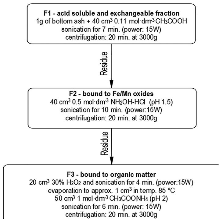
**Figure 2.** The BCR sequential extraction procedure
