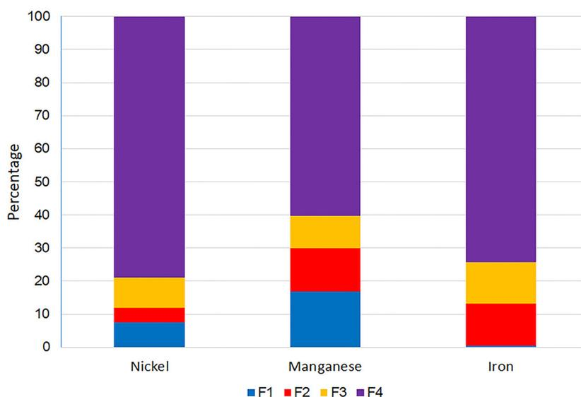
**Figure 3.** Fractions of Ni, Mn and Fe in bottom ash
