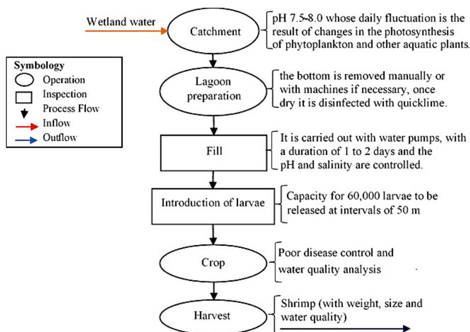
Figure 2. Diagram of the shrimp production process
