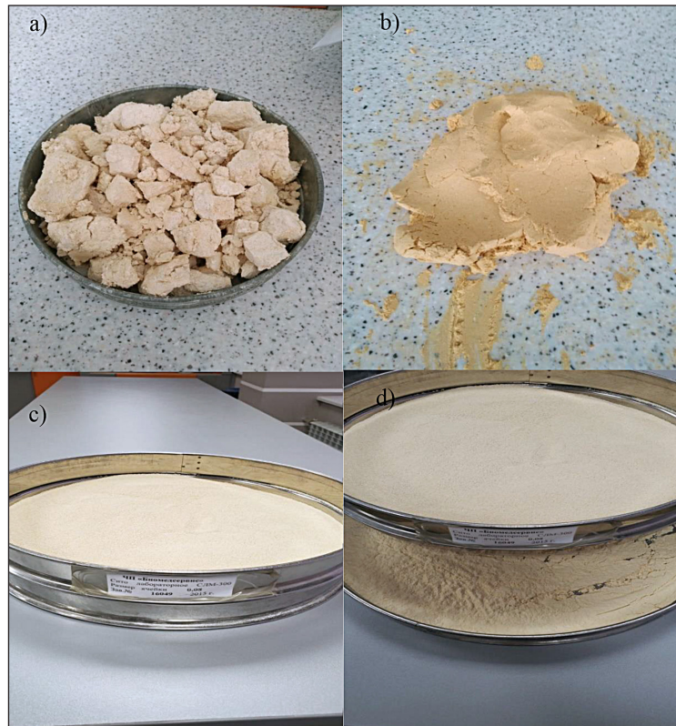
Figure 3. Production of bentonite clay powder
