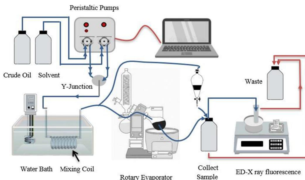
**Fig. 1.** 2D Graphic of semi-automated flow injection system – X-ray system
