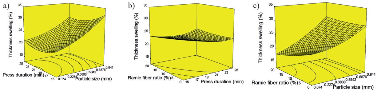
**Figure 2.** Response surface 3D plots on thickness swelling of hybrid bio panels (a) particle size and press durations, (b) ramie fiber ratio and press durations, and (c) ramie fiber ratio and particle size
