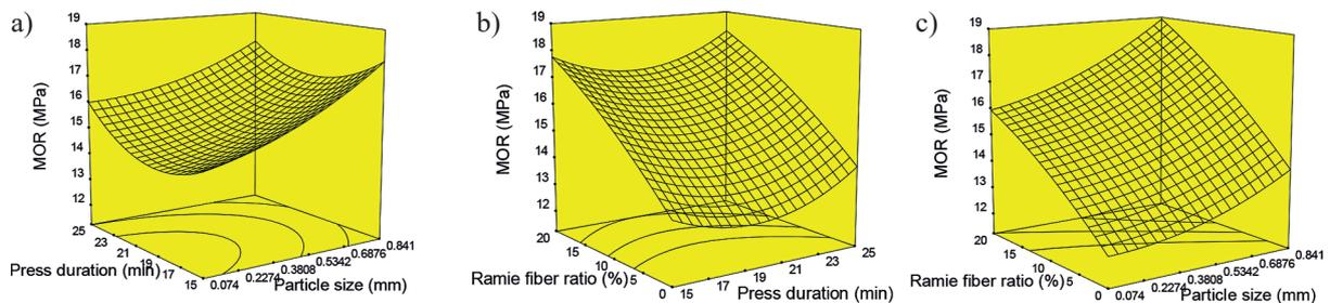
**Figure 3.** Response surface 3D plots on MOR of hybrid bio panels (a) particle size and press durations, (b) ramie fiber ratio and press durations, and (c) ramie fiber ratio and particle size
