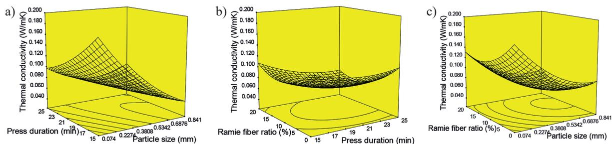
**Figure 4.** Response surface 3D plots on thermal conductivity of hybrid bio panels (a) particle size and press durations, (b) ramie fiber ratio and press durations, and (c) ramie fiber ratio and particle size
