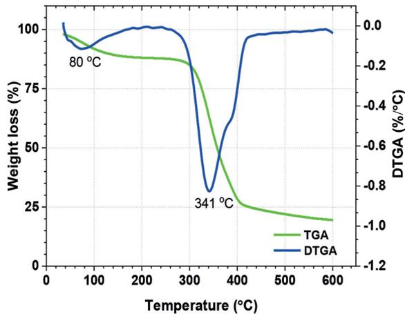
Figure 5. TGA and DTGA curve of hybrid bio-panels based on OPT
