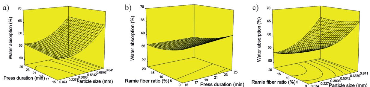
**Figure 1.** Response surface 3D plots on water absorption of hybrid bio panels (a) particle size and press durations, (b) ramie fiber ratio and press durations, and (c) ramie fiber ratio and particle size
