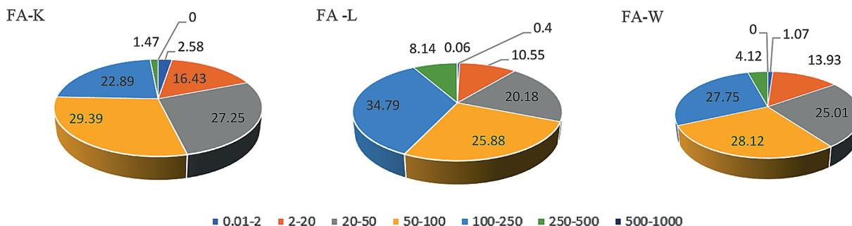
Figure 3. Volumetric distribution of individual particle fractions in the investigated ashes
