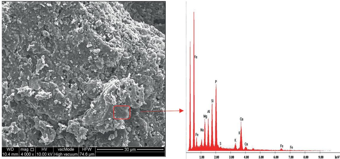
Figure 5. SEM photos of the tested ash from Łódź together with the EDS analysis
