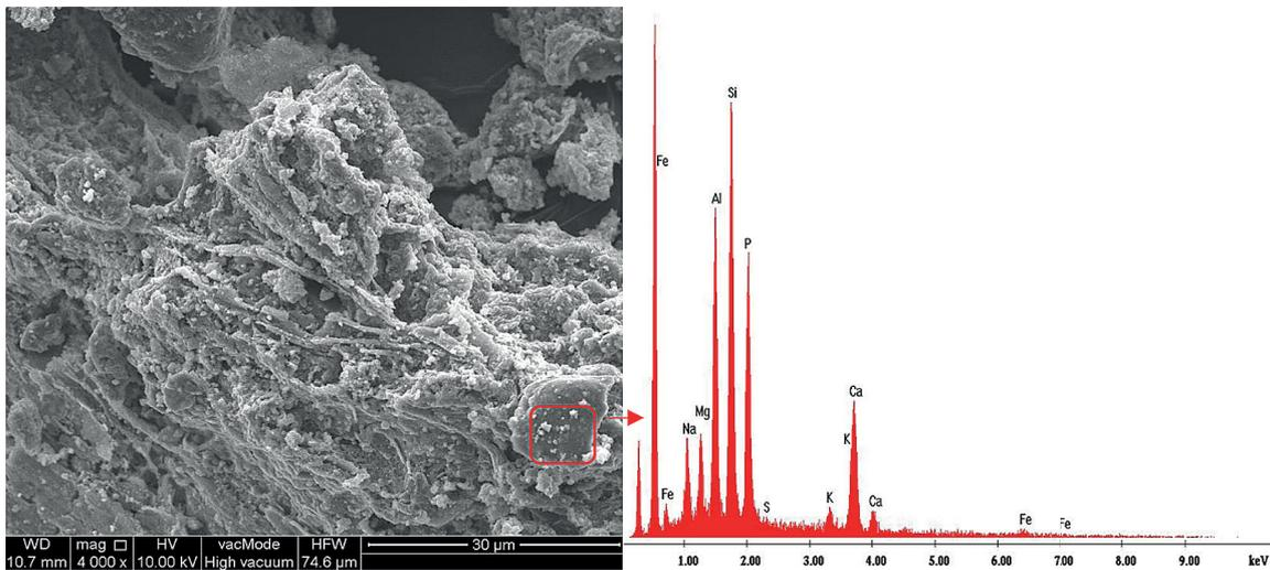
Figure 6. SEM photos of the tested ash from Warsaw together with the EDS analysis
