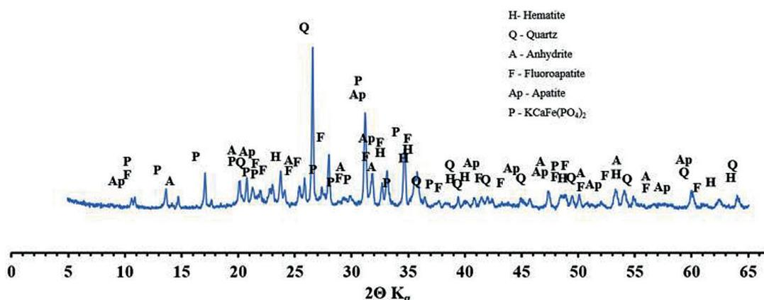
Figure 7. XRD pattern of the applied sludge fly ash
