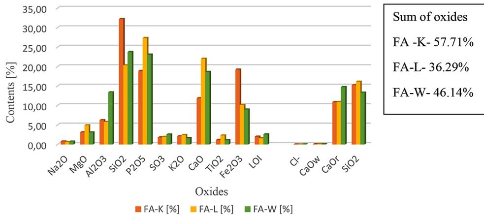
Figure 1. Chemical composition of fly ash from sewage sludge
