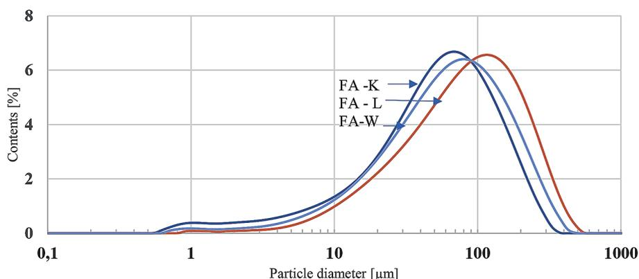
Figure 2. Particle size distribution curve in the tested fly ash
