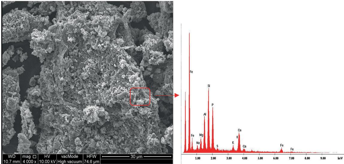
Figure 4. SEM photos of the tested ash from Cracow together with the EDS analysis
