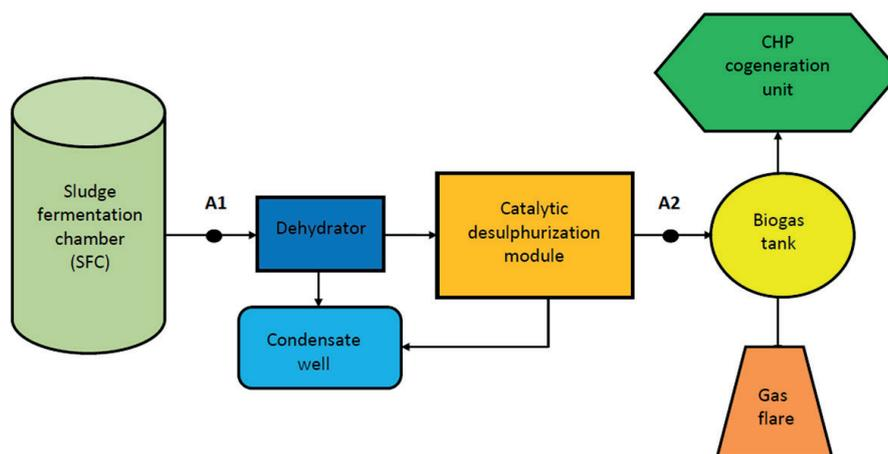
**Figure 1.** Technological flowchart of type A biogas conditioning installation
