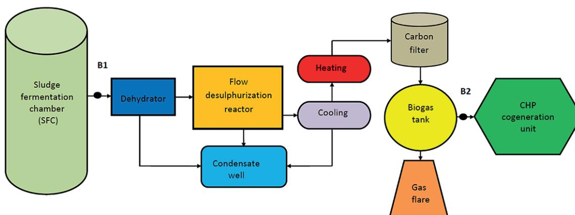
**Figure 2.** Technological flowchart of type B biogas conditioning installation
