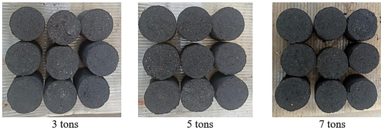
**Figure 3.** Physical appearance of the rice husk charcoal briquettes with a compacting pressure of 3 tons, 5 tons and 7 tons
