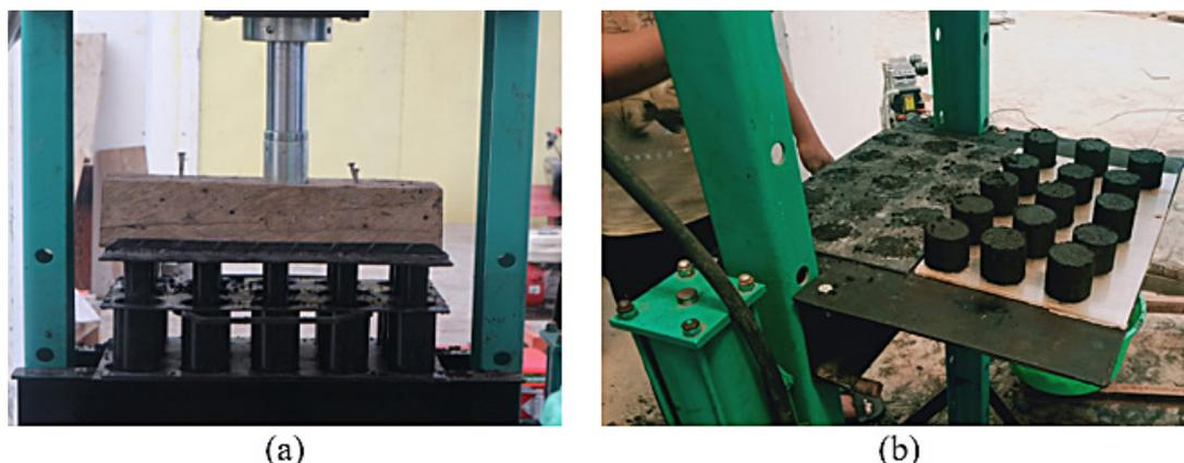
**Figure 2.** One of the stages of making briquettes: (a) dough pressing; and (b) printed briquettes
