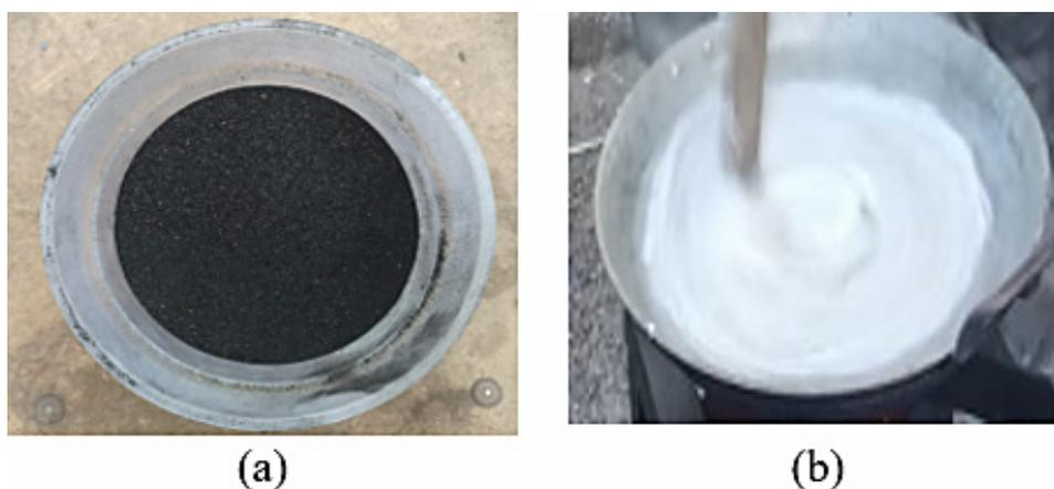
**Figure 1.** Briquette dough ingredients: (a) rice husk powder and (b) adhesive mixtures
