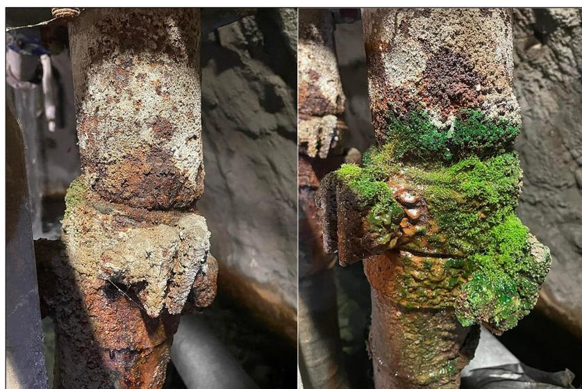
**Fig. 6.** Flora developing on corrosion products under 24h white light illumination. Level 640, drainage of Jurassic formations. (Photo: M. Ciosmak)
