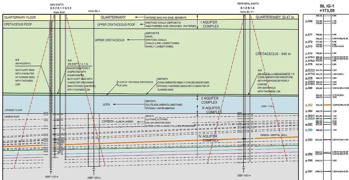
Fig. 2. Geological profile of the mining area (Source: LW “Bogdanka” S.A.)
