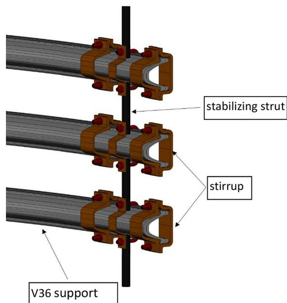
Fig. 3. Elements of the V36 type excavation support
