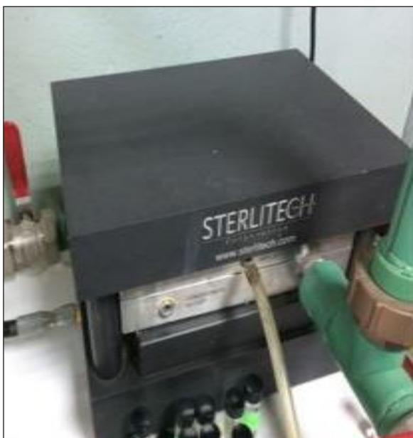
Figure 2. NF and RO membranes cell
