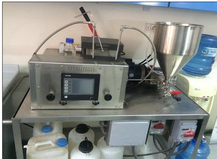
**Figure 4.** Bench scale of flat plate RO membrane filtration system
