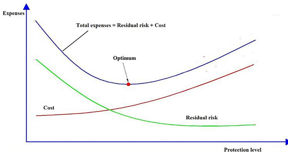
Fig. 3. Optimal protection level
