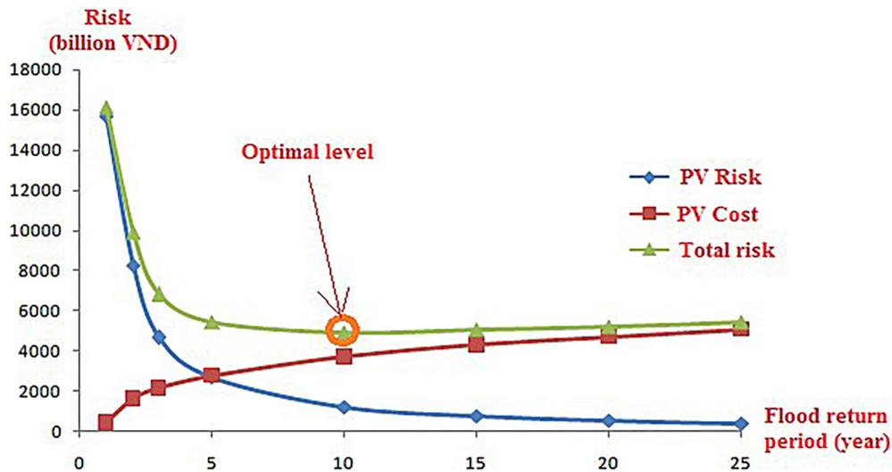
Fig. 4. Optimal protection level using the discrete method
