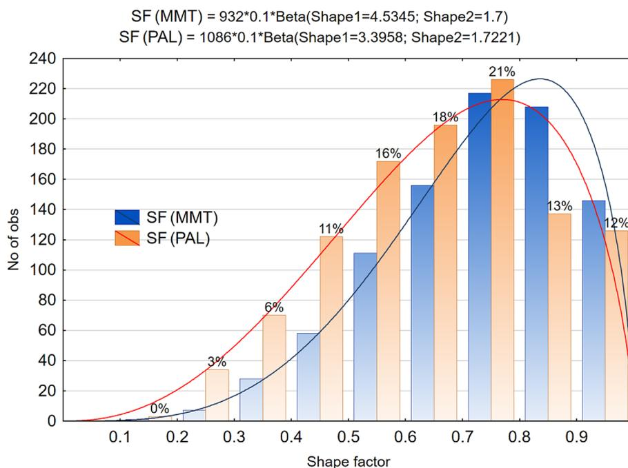
Figure 3. Distribution of MMT and PAL clay particles by shape factor
