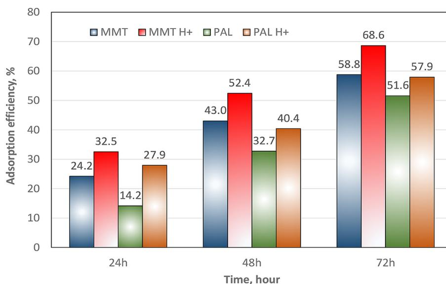
**Figure 8.** Adsorption efficiency of clays before (MMT, PAL) and after (MMT H<sup>+</sup>, PAL H<sup>+</sup>) acid activation
