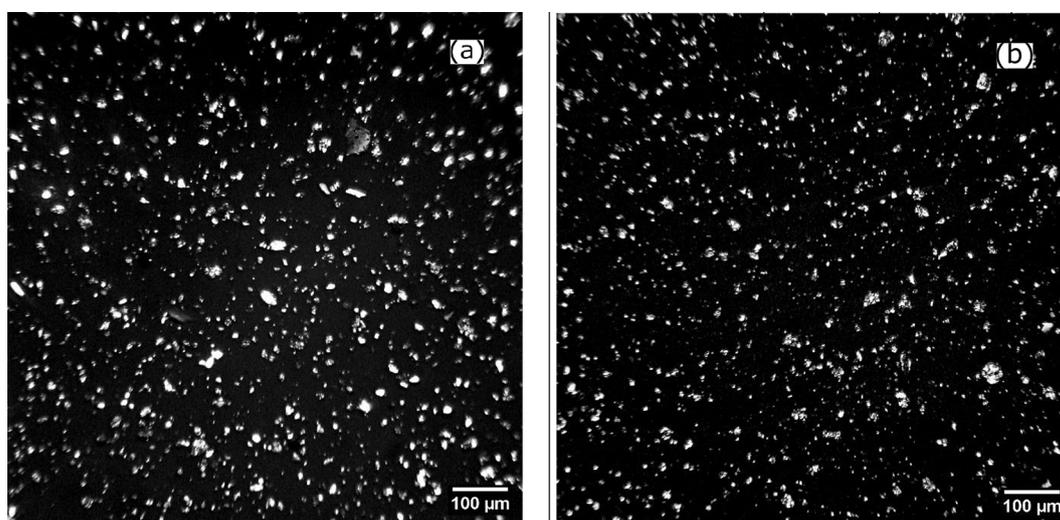
**Figure 1.** Micrographs in polarized light of clay particles of MMT (a) and PAL (b) samples
