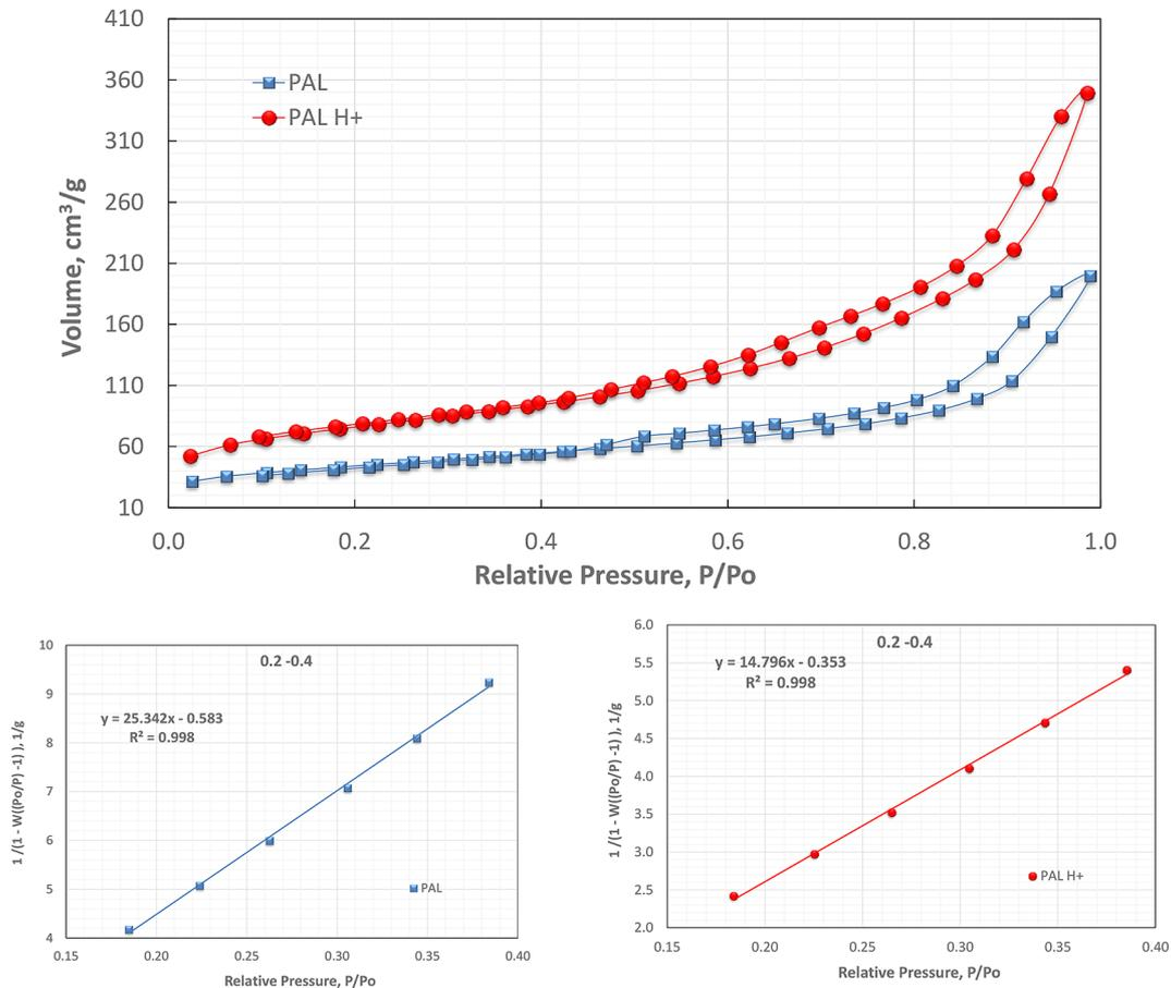
Figure 5.  $N_2$  adsorption isotherms of pure and acid activated PAL (a) and linear fitting plots (c, d) of multi-point BET isotherm models
