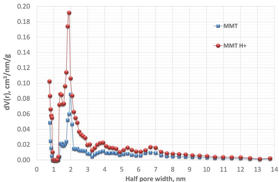
Figure 6. Pore size distributions in montmorillonite (DFT method) before (MMT) and after (MMT H<sup>+</sup>) acid activation
