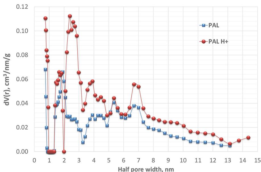
**Figure 7.** Pore size distributions in palygorskite (DFT method) before (PAL) and after (PAL H<sup>+</sup>) acid activation
