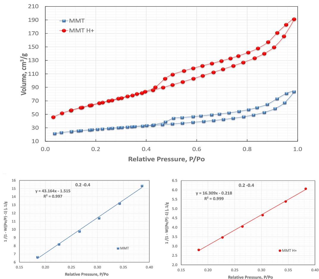
**Figure 4.**  $N_2$  adsorption/desorption isotherms of pure and acid activated MMT (a) and linear fitting plots (b, c) of Multi-Point BET isotherm models
