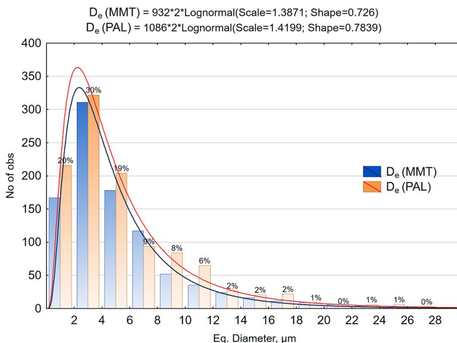
**Figure 2.** Distribution of MMT and PAL clay particles by equivalent diameter
