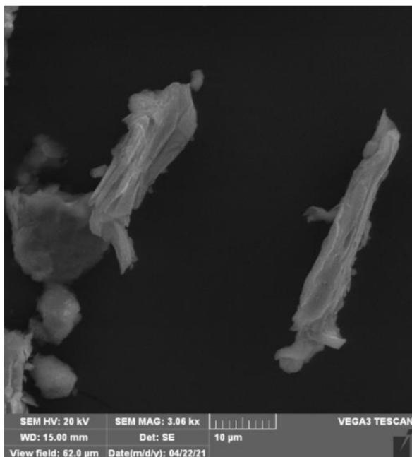
**Figure 2.** The results of SEM analysis using pictures of Brari clay with a resolution 10 μm
