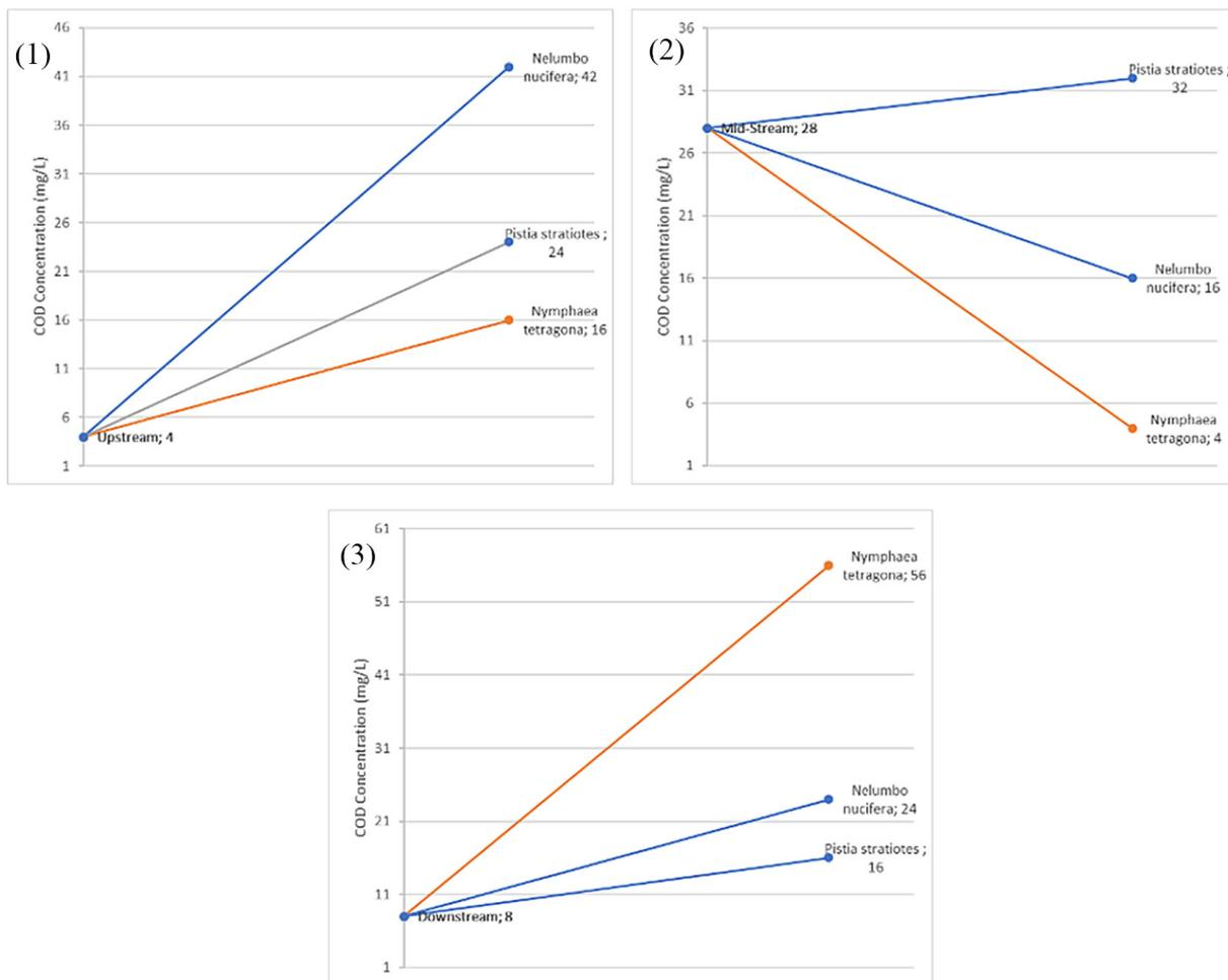
**Figure 5.** The COD concentration in each effluent of candung from upstream (1), mid-stream (2) and downstream (3)
